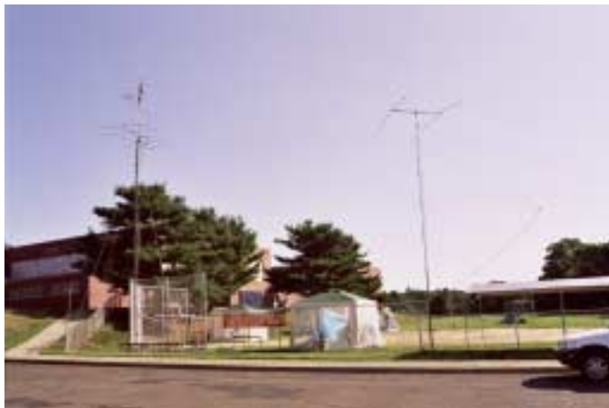
The Antennas at Governor Livingston. 20 Meter Yagi on the right and VHF arrays on the left.
