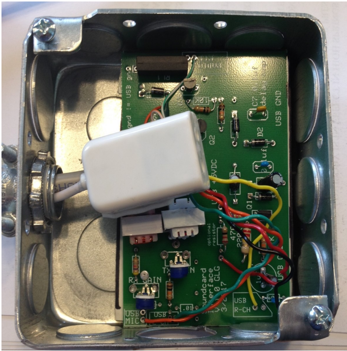
Figure 3-3. Printed circuit board mounted (actually wedged) into a 4” electrical box. One knockout has been removed to allow access to the potentiometers, The USB dongle is also inserted, and another knockout has been
