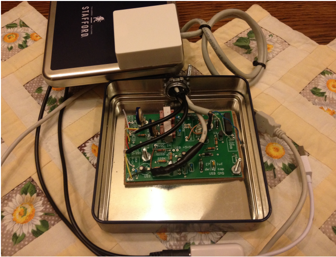
Figure 3-1. Mounted using screws to a left-over metal box. A layer of 1/4" spare wood paneling was used as an insulator to protect the solder connections from shorting out to the metal box. The attractive metal box was the packaging of a nice man's wallet received as a Christmas present. Electrician's 1/2" non-metallic cable clamp is used to secure and protect the cables passing through hole
