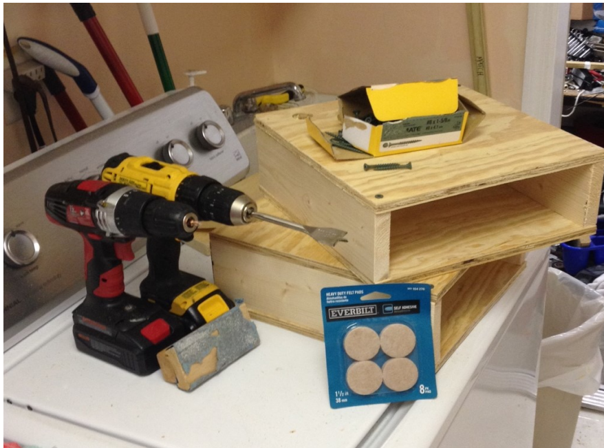
Figure 3. Screwing the boxes together. It is a lot easier if you have more than one drill, so you don't have to keep switching tools.
