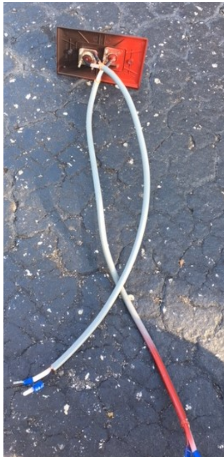
Figure Two: Nylon face plate with top end marked RED and top cable marked with RED paint.
