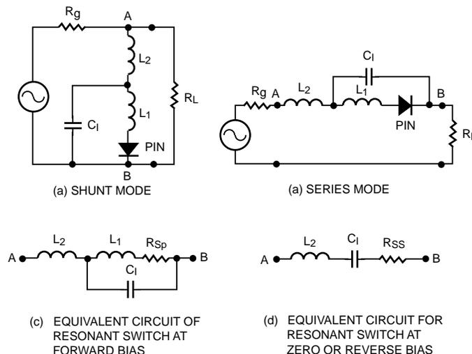
**Figure 12. Resonant PIN Switch Circuits.**
