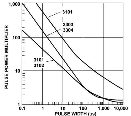
Figure 26. Pulse Power Multiplier vs. Pulse Width.
