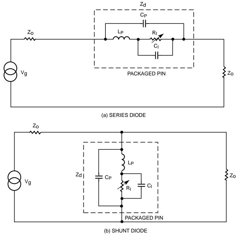
Figure 9. Packaged Diodes Used as Reflective Attenuators.
