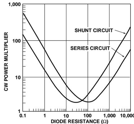
Figure 23. CW Power Multiplier vs. Diode Resistance.
