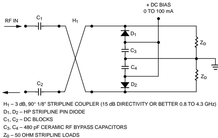
Figure 17. S-Band Single Hybrid Coupled PIN Attenuator.
