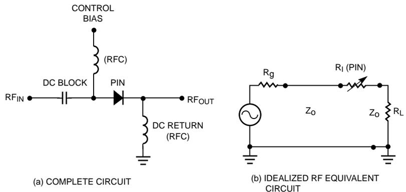
Figure 7. Series PIN RF Attenuator or Switch.
