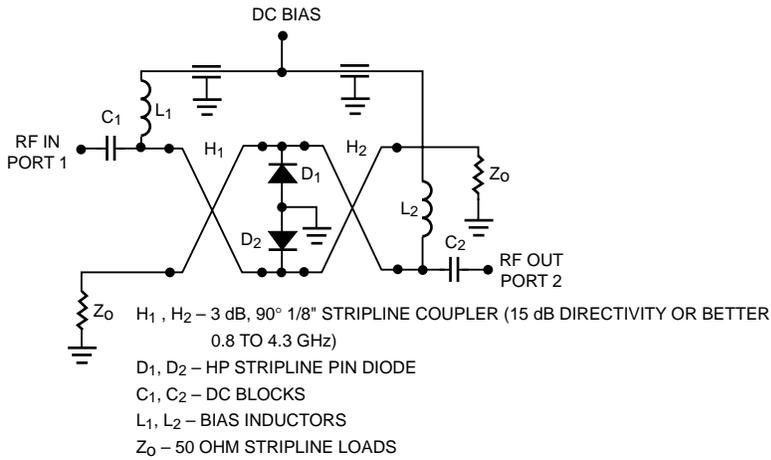
Figure 20. S-Band Double Hybrid Coupled PIN Attenuator.
