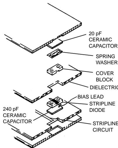
Figure 19. PIN Diode Biasing in Stripline Structures.
