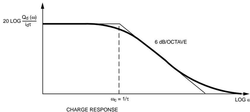
Figure 1. PIN Behavior as a function of Frequency.
