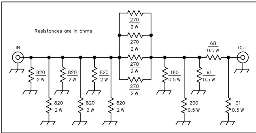
Figure 16—A 20-W, 20-dB attenuator for transmitter measurements.
