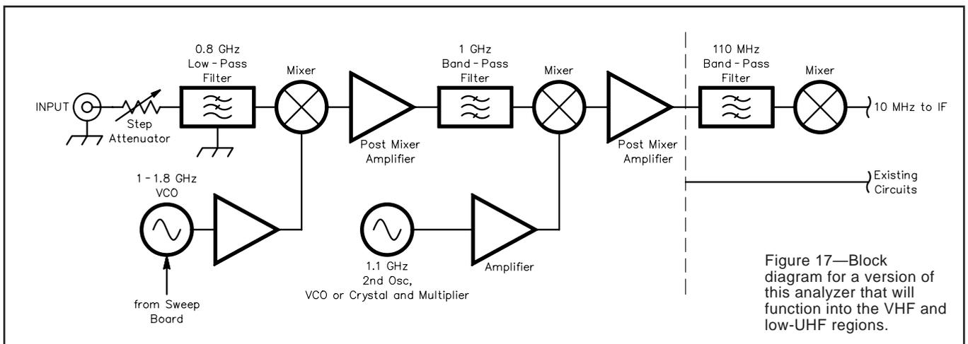
Figure 17—Block diagram for a version of this analyzer that will function into the VHF and low-UHF regions.
