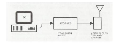
Figure 1-2: Amateur Paging System 2-meters or 70-cm.
