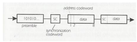
Figure 3-3: Two-Way POCSAG QSO Transmission
