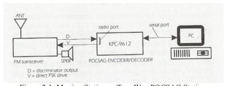
Figure 3-1: Monitor Station or Two-Way POCSAG Station
