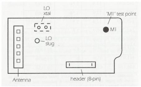
Figure 6-1: VHF Receiver Board AARD405X Series
