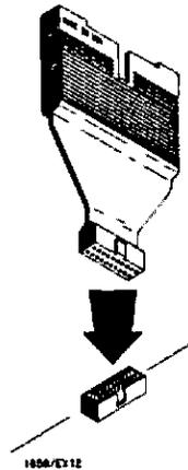
Figure 12-2 Termination Adapter
