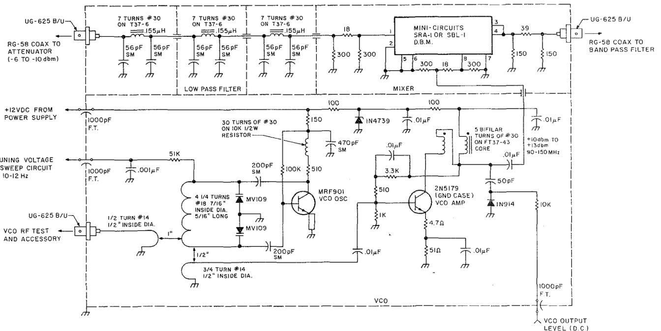
Note 1. Resistors are 1/4 W, 5%; unspecified capacitors are 50-V ceramic.
