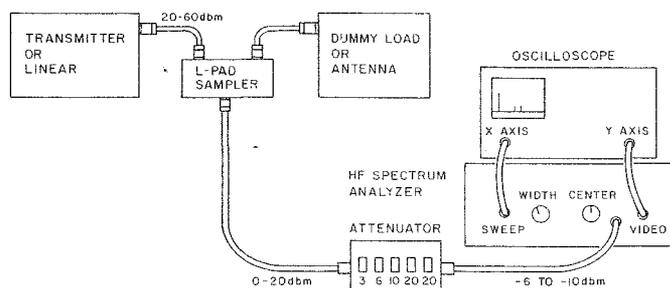
Note 1. Never hook transmitter or linear directly to step attenuator or analyzer. Always use L-pad sampler of the proper power rating.
