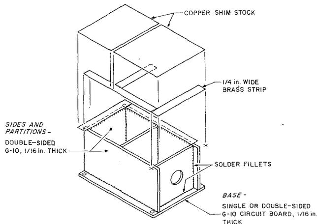
Note 1. Solder G-10 circuit board and brass strips with 40-W iron.
