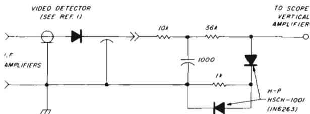
fig. 2. Signal-processor circuit as modified by N6TX for use with his microwave spectrum analyzer.<sup>1</sup>
