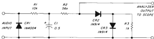
fig. 1. Pseudo-logarithmic signal-processing circuit developed by W3JW for use in a high-frequency spectrum analyzer.<sup>2</sup>
