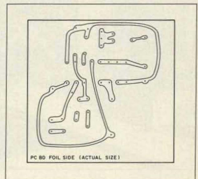
Figure 2. Foil side of board, actual size.
