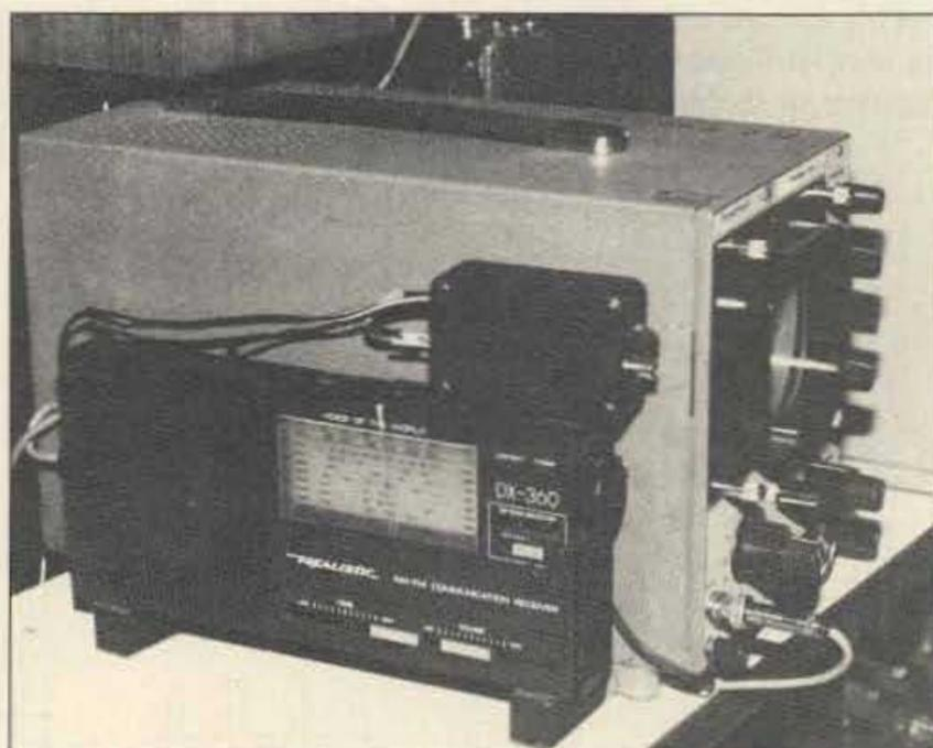
Photos C,D. Greg KE0UV getting ready to to spot some DX on 10m using the \$10 Spectrum Analyzer. Photo D is a close-up of the system, comprised of the o'scope, the scanning receiver (the DX-360) and the interface, which sits atop the DX-360.
