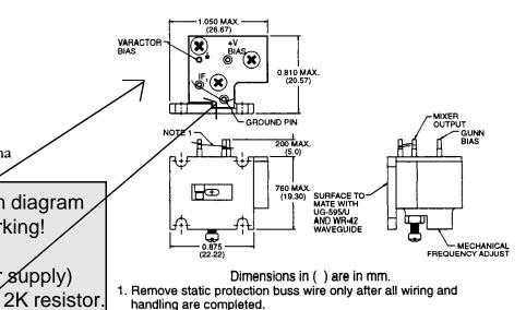
The MA87729-MO1 transceiver can be factory modified to operate at other frequencies close to 24.150 GHz if required to meet the allowed frequency requirements of countries other than the US. These transceivers can be factory modified to have other electronic tuning ranges and/or to have a negative tuning voltage.
