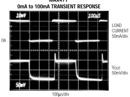
$V_{CC}$  = 10V,  $R_{OUT}$  = 2k $\Omega$  1%, SIGN PULL-UP = 50k $\Omega$  1%
