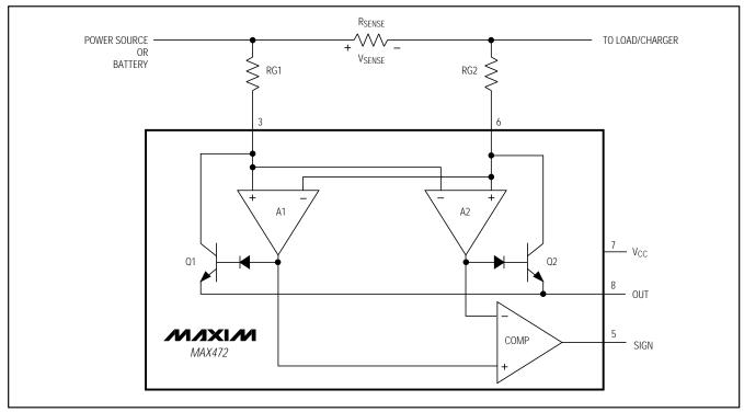
Figure 2. MAX472 Functional Diagram
