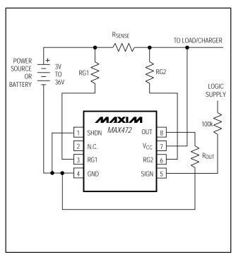
Figure 4. MAX472 Standard Application Circuit
