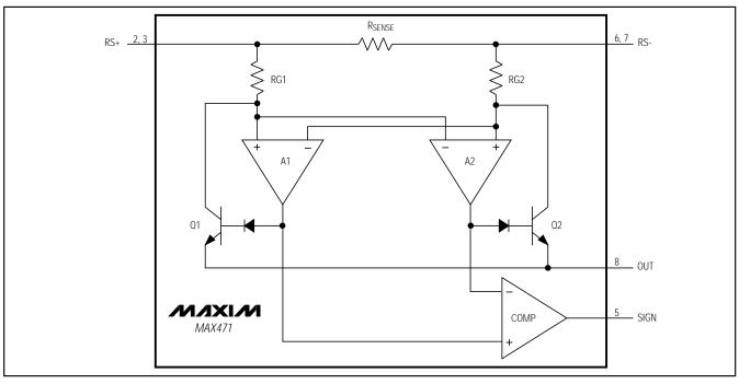
Figure 1. MAX471 Functional Diagram
