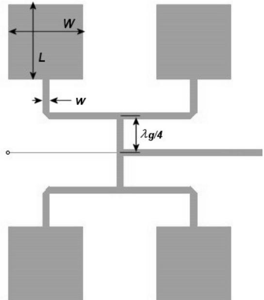
Fig. 1. Typical microstrip phased array antenna.
