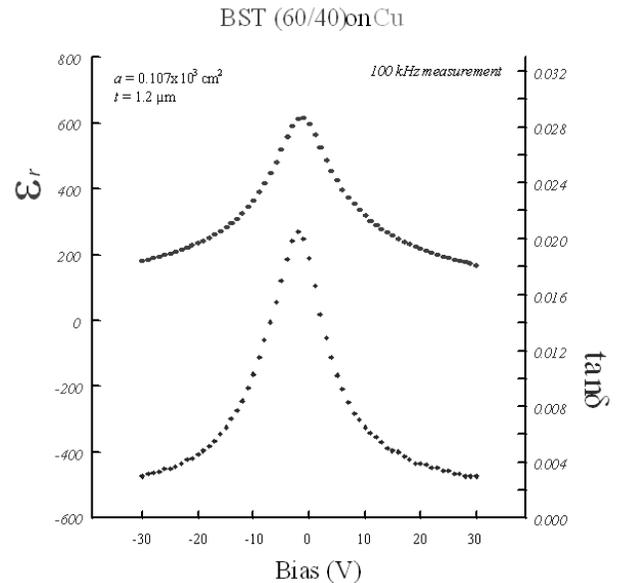
Fig. 2. C/V and Loss Tangent curves for typical ferrotunable material.
