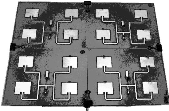
Fig. 7. Varactor-tuned test array on conventional substrate.
