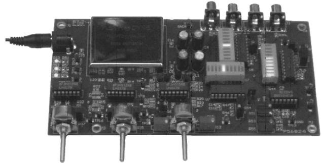
Fig. 8. Analog test fixture for limited frequency tuning and beam steering.
