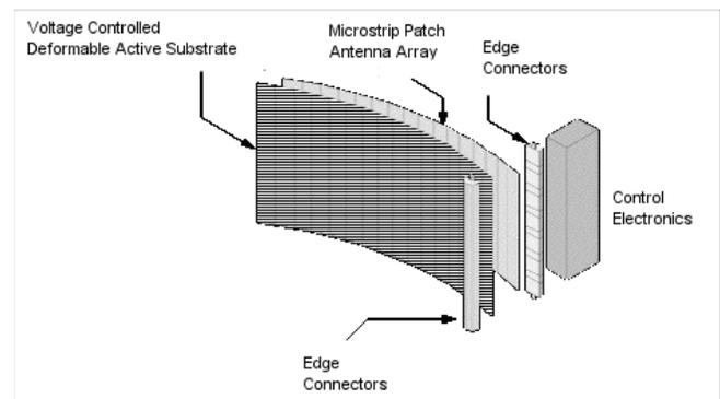
Fig. 6. Use of active substrate for antenna steering.
