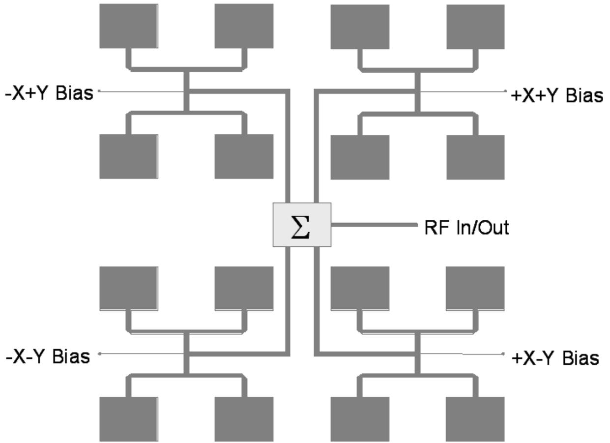
Fig. 3. Quadrant steering of microstrip patch array.
