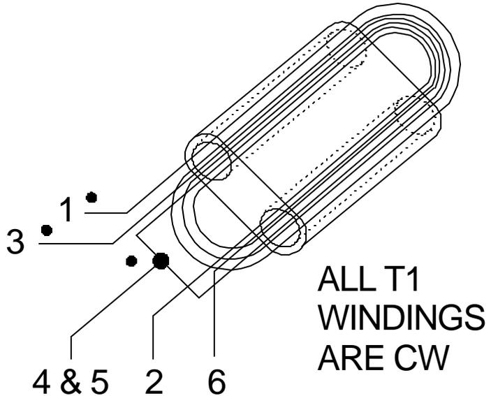
1. Orient core as shown above. All windings in T1 are CW. 1 pass through BOTH holes = 1 TURN. Wind 4T
