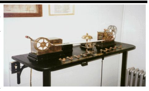
improvement was a series of contacts and wipers that would decipher the particular station's code and sound an alarm bell.
