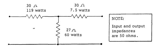
For Linears Requiring 12 Watts Drive
