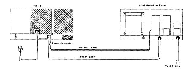
FIG.1 CONNECTING THE TR-4 TO THE AC-3 POWER SUPPLY AND MS-4 MATCHING SPEAKER
