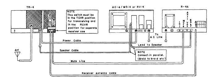
FIG. 3 USING THE TR-4 WITH AN EXTERNAL RECEIVER
