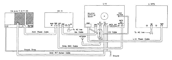
FIG 21 CONNECTING THE TR-3/TR-4/T-4X AND AC-4 TO THE L-4 LINEAR AMPLIFIER
