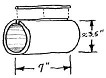
THIS PIPE WILL BECOME THE COIL FORM. PULLING THE WIRE OUT OF THE SLOT ALLOWS THE FORM TO SHRINK IN DIAMETER, RELEASING THE COIL WHEN IT IS FINISHED.
