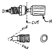
CUT SHANK OF 5-WAY BINDING POST THROUGH HOLE & THREAD PLASTIC HEAD OFF OF JACK PORTION, -HEAD LEAVING FEMALE SOCKET WITH GROOVED END.
