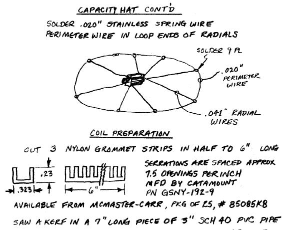
AND WEDGE A SECTION OF 14 GAUGE WIRE IN THE KORF
