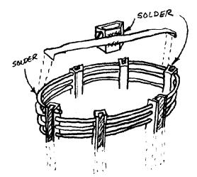
CUT A "18 OR "116" DIAMETER PIECE OF COPPERHOBBY TUBING TO A LENGTH SLIGHTY LONGER THAN COIL DIAMETER. FLATTEN THE ENDS & FORM LIPS TO FIT OVER TOP TURN OF COIL. SOLDER ANOTHER COPPER GROUND LUG CLIP TO DAR & SOLDER BAR TO TOP TURN OF COIL.
