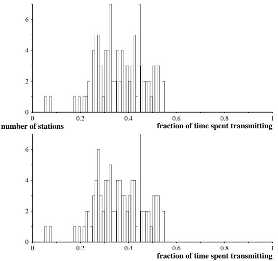
Figure 4.6: Distributions of the transmit duty cycle. The top is without the respectneighbor constraint, and the bottom is with the respect-neighbor constraint. There are no significant differences between the transmit duty cycles with and without the respect-neighbor constraint.
