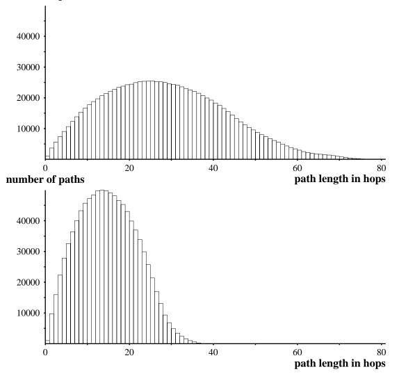
Figure 5.5: Distribution of path lengths of the 1,000,000 different paths in the network of 1,000 stations. The top plot is for minimum energy routes. The bottom plot is for the paths produced by the modified routing computation.
