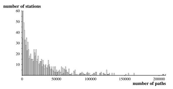
Figure 5.1: Distribution of number of paths routed through each station in the network of 1,000 stations using minimum energy routes (as shown in Figure 4.9). For each source-destination pair there is one path, for a total of 1,000,000 paths.
