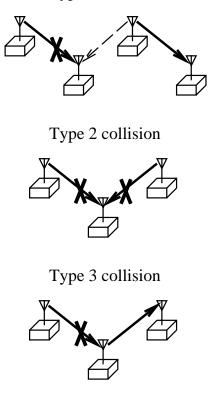
Figure 2.2: Examples of each type of collision. The X indicates the lost packet.
