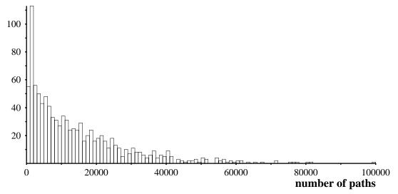
Figure 5.6: Distribution of number of paths routed through each station in the network of 1,000 stations using routes produced by the modified routing computation.
