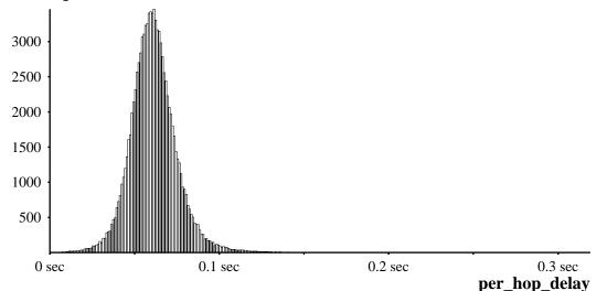
Figure 5.9: Distribution of measured end-to-end delays divided by number of hops, or the average per-hop delay, experienced by each packet in a lightly-loaded 1,000-station network with minimum energy routes, 64 slots per second, and 16 subslots per slot.
