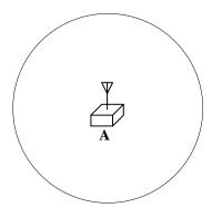
If the most distant stations we are communicating with are at a distance of  $2\rho^{-\frac{1}{2}}$ , then the expected number of stations inside a circle with a radius of one-fifth this distance is only  $\pi \left(\frac{2}{5}\right)^2 \approx 0.5$ . This number is well under the interference threshold of 4 nearby transmitters selected above. Therefore this form of interference will not often be a problem.
