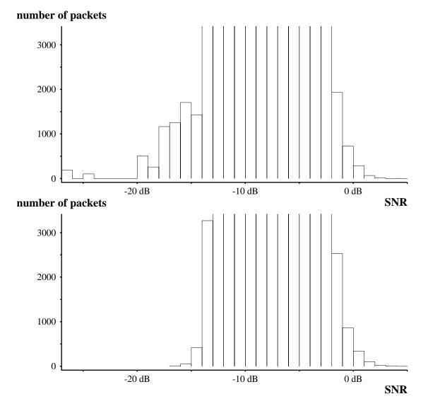
Figure 4.8: Same as Figure 4.7 but at a magnified vertical scale so that the tails can be seen more clearly. In the bottom distribution (for the case with the respect-neighbor constraint) no packets were received with a signal-to-noise ratio of less than -17 dB.
