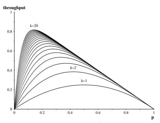
Figure 3.3: Variation of throughput,  $(1-p) - (1-p)^{k+1}$ , with receive duty cycle, p, for the number of neighbors k ranging from 1 to 20. Note that p near 0.3 produces good throughput for a wide range of k.
