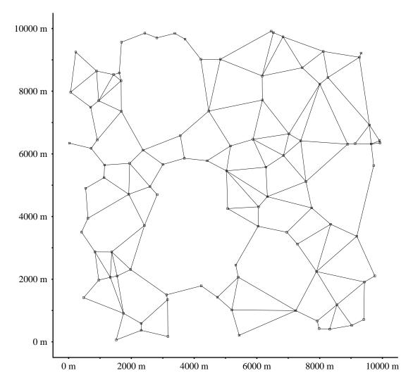
Figure 4.2: Direct hops used by minimum-energy routes.
