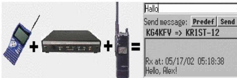
Composite screen shot: Left - basic Cybiko APRS station components Right - screen shot from Cybiko PDA running UI Messenger.
