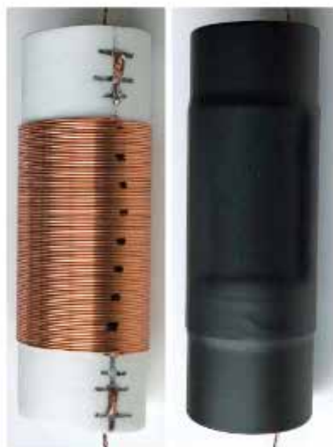
▲ Figure 2 — On the left, the loading coil is shown uncovered, and the right image shows it covered with heat shrink.
