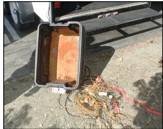
This is why we do a preliminary check. No one expected our wire antennas to get left out in the rain. Note the rust stain on the storage container.
