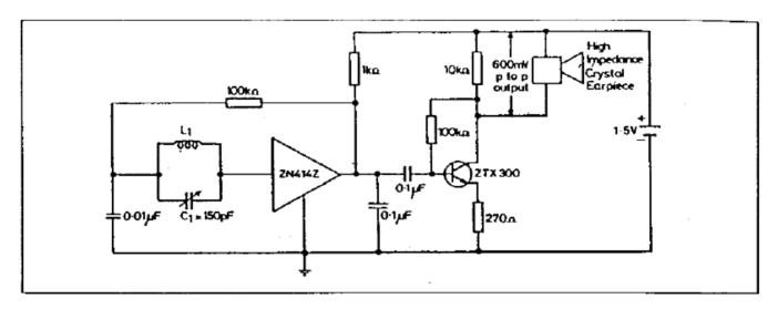
Li =80 turns of 0.3mm dia. enamelled copper wire on a 5cm or 7.5cm long ferrite rod. Do not expect to adhere rigidly to the coil-capacitor details given. Any value of  $L_1$  and  $C_1$  which will give a high 'Q' at the desired frequency may be used. Volume Control: a 250 $\Omega$  potentiometer in series with a 100 $\Omega$  fixed resistor substituted for the 270 $\Omega$  emitter resistor provides an effective volume control.
