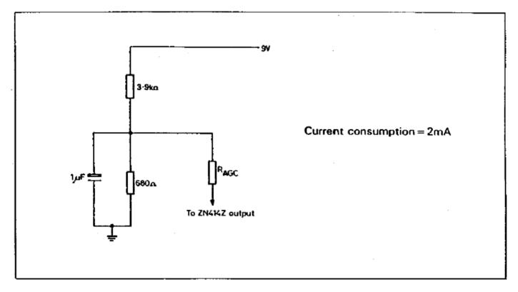
Note: Replacing the  $680\Omega$  resistor with a  $500\Omega$  resistor and a  $250\Omega$  preset, sensitivity may be adjusted and will enable optimum reception to be realised under most conditions.
