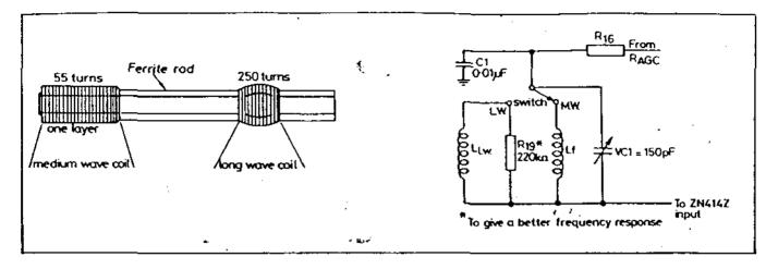
Coil winding details and waveband selection
