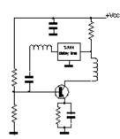
A SAW delay line can be used to effect in the circuit shown. The various reactive components ensure a 180 degree phase shift between input and output. No part values are given, as these depend on actual unit used and layout.
