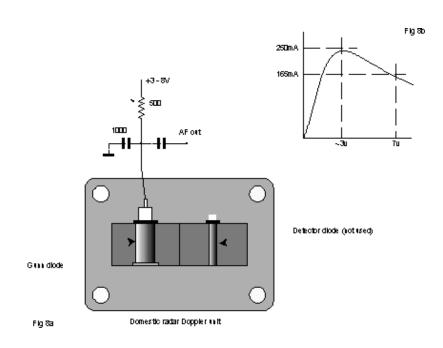
Another interesting application showing the use of a domestic radar Doppler module as a very sensitive 10GHz receiver. Using another module as the transmitter, range can be several tens of meters. The mixer diode is not used in this instance.
