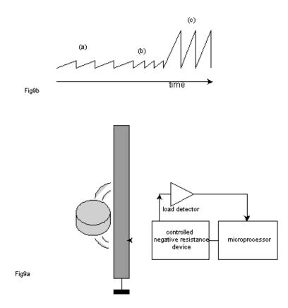
A concept for a micro miniature code device or transponder. A Dielectric resonator bead is coupled to a resonant cavity or micro strip line to stabilise its operating frequency. Controlled negative resistance bursts are applied at low level (a), when acting as a sampled time receiver, and at high level (c) when acting as a transponding reply radiator.
