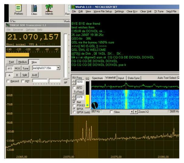
$\underline{\text{test 1}}$  Connect the antenna to the receiver, read the noise floor level. Disconnect the antenna and read the noise level again. If the level is the same (here is the same) the total receiver gain is not sufficient. The noise that you view in the screen is internal receiver noise, not atmospheric noise.
