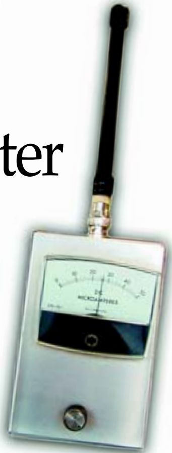
The RF Signal Strength meter responding to my Kenwood TH-26AT transmitting on 147.900 MHz with 1 W, 2 feet away from the meter. The sensitivity control is set at mid range.
