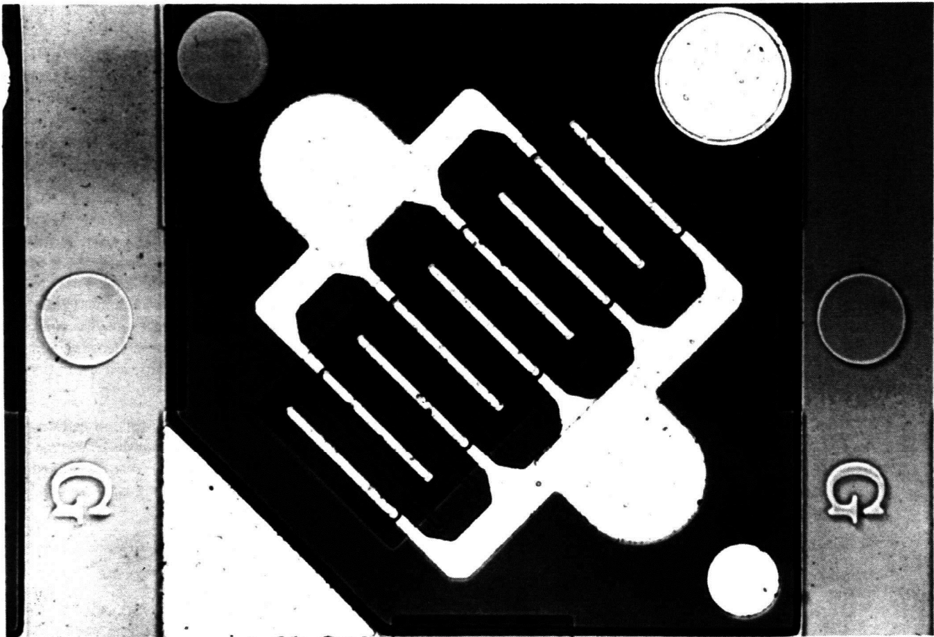
Figure 1. A Junction Field Effect Transistor (JFET). One of the JFETs used in the FETRON, and in volume production for high reliability missile systems and many other applications.
