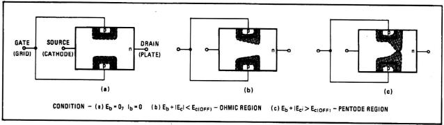
1. **Brothers.** JFET's elements are analogous to tube elements. The JFET source is comparable to the cathode, its drain to the plate, and gates to the grid. As the grid (plate) voltage goes negative, plate (drain) current drops. The gate's p-regions, growing into the channel, causes pinchoff, which is analogous to tube's cutoff.
