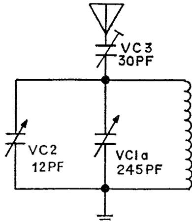
Figure 10 Tuning Circuit for Short Wave Bands, Simplified
