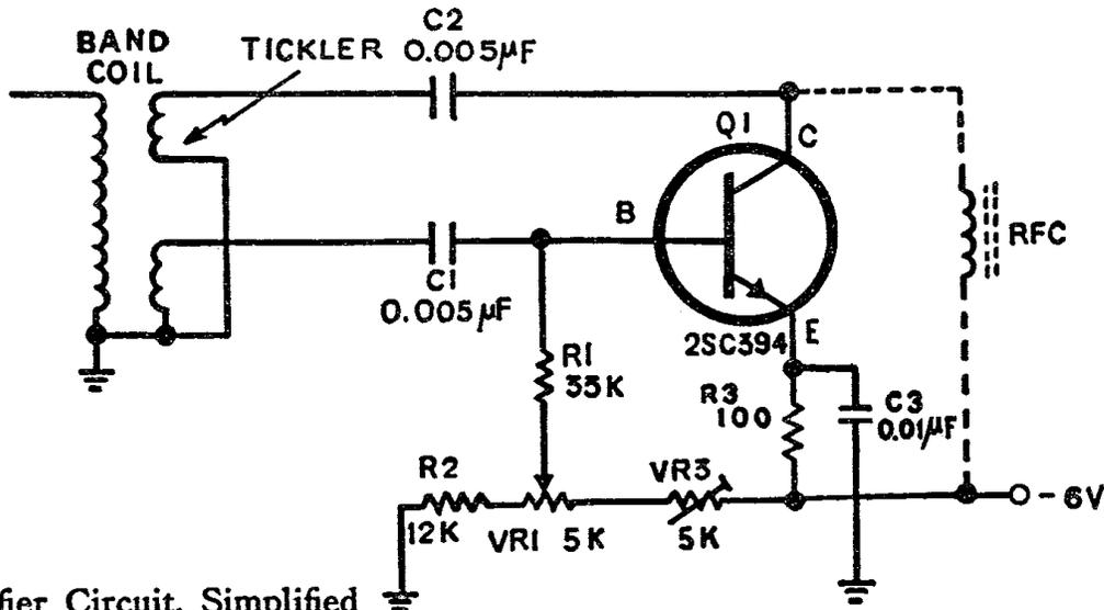
Figure 11 RF Amplifier Circuit, Simplified
