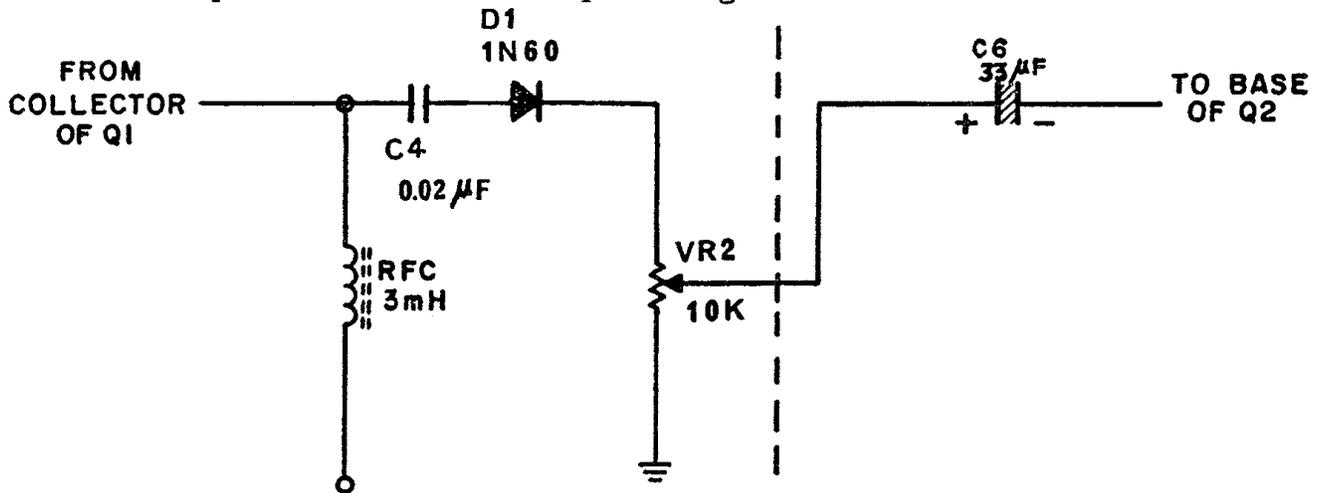
Figure 12 Detector Circuit, Simplified
