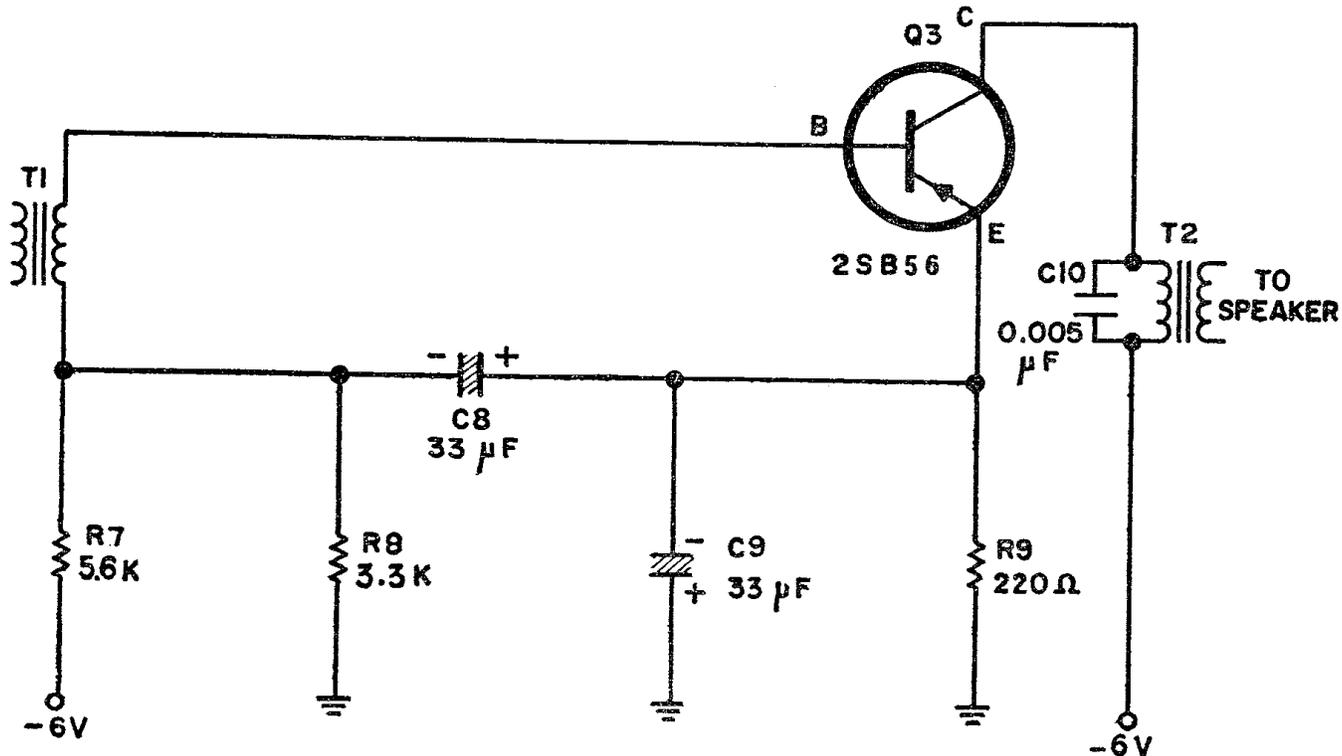
Figure 14 Power Output Stage, Simplified
