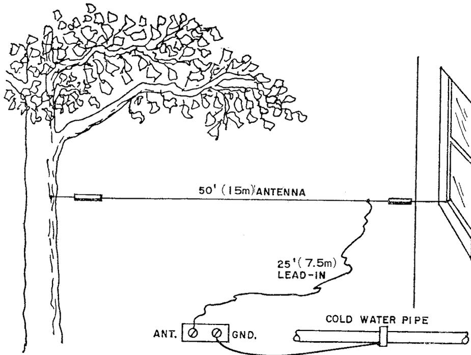
Figure 7 External Antenna for Globe Patrol Receiver
