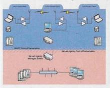
Due to the 6 to 54 megabit bandwidth, multiple simultaneous communications can take place on a single channel. Any site can act as an intelligent digital repeater into the network and thereby expand the mesh, provided it has proper credentials.
