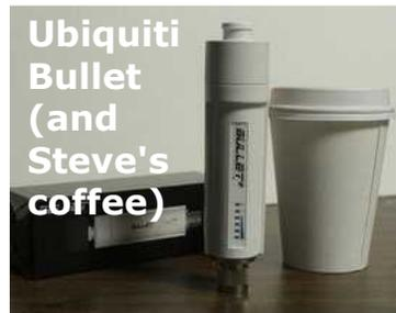
Another option if you need an external antenna is Ubiquiti's 2.4 GHz bullet. It's their simplest, and cheapest (\$40) 802.11 device. It's basically a ethernet->N converter that allows you to connect an external antenna.
