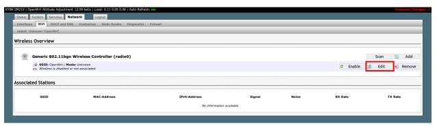
Press the "Edit" button to enter additional configuration data for the wifi interface. NOTE: If you are configuring a device with multiple radio cards/ports, this configuration applies to the 2.4GHz card/port you desire to attach to the mesh.
