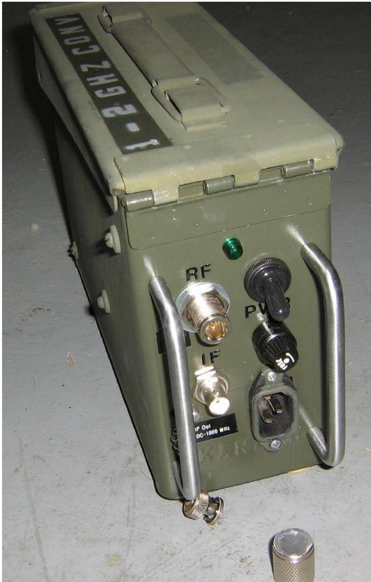
The 1–2 GHz RF input is via the panel–mount N connector.
