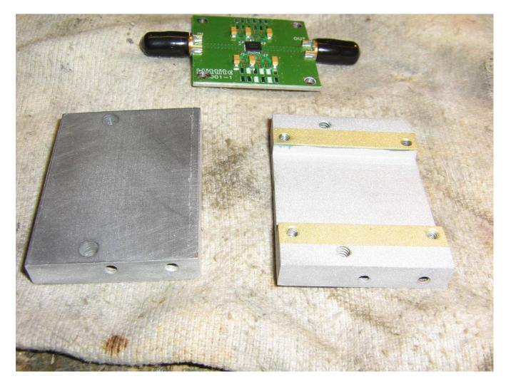
Overview of the Hittite HMC487 evaluation board and the milled aluminum mounting block.
