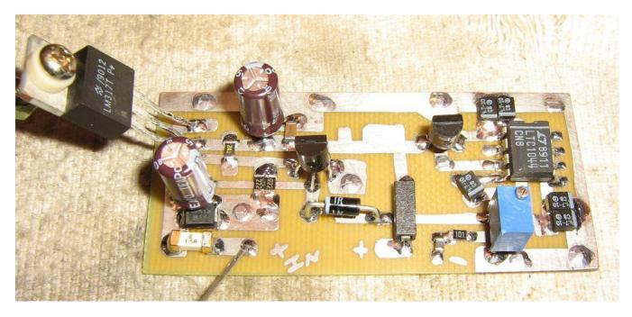
Overview of the Hittite HMC487 evaluation board power supply circuit.
