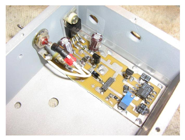
Installing the power supply circuit in the project box.
