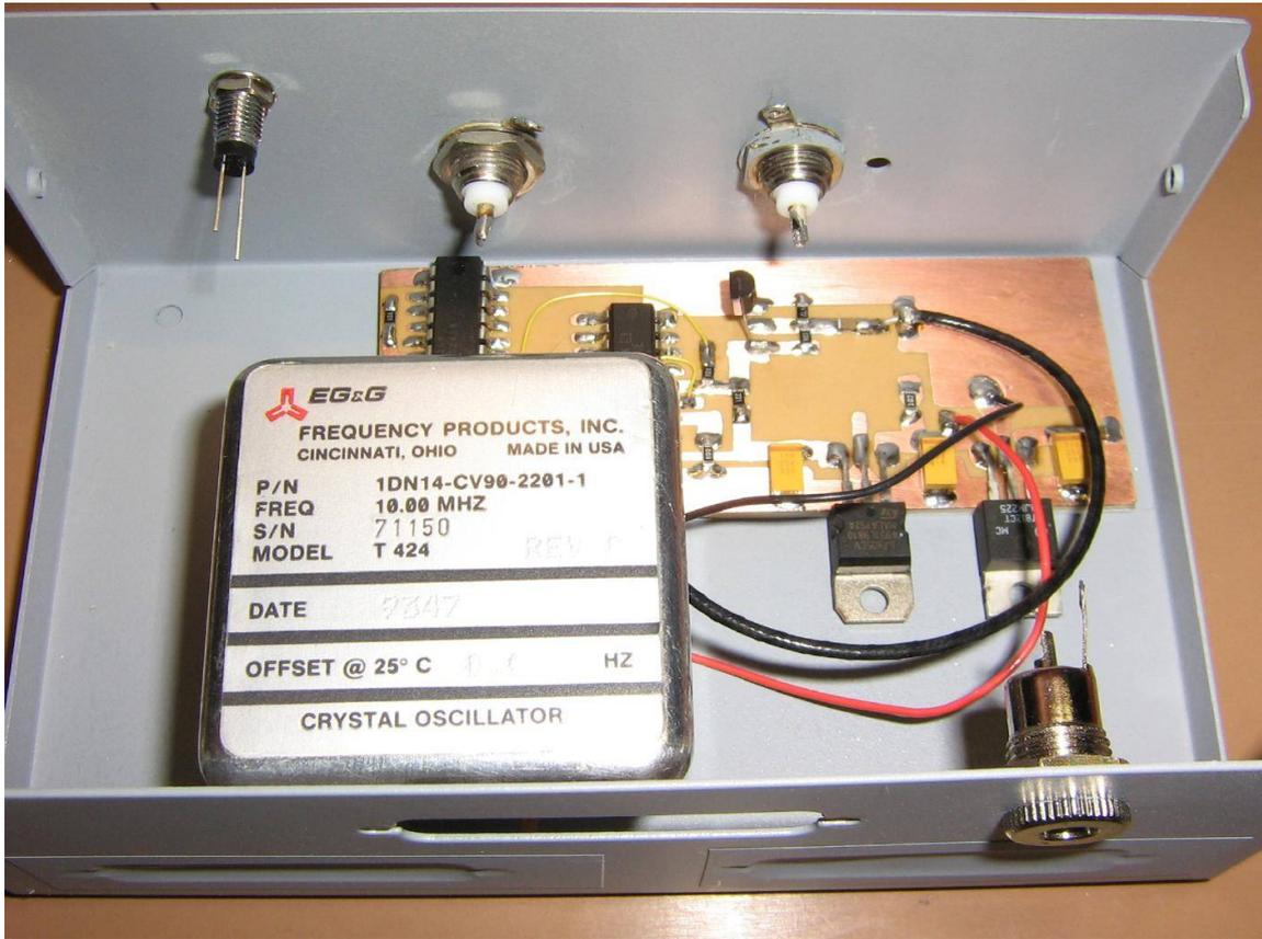
Mounting the oscillator and circuit board.
