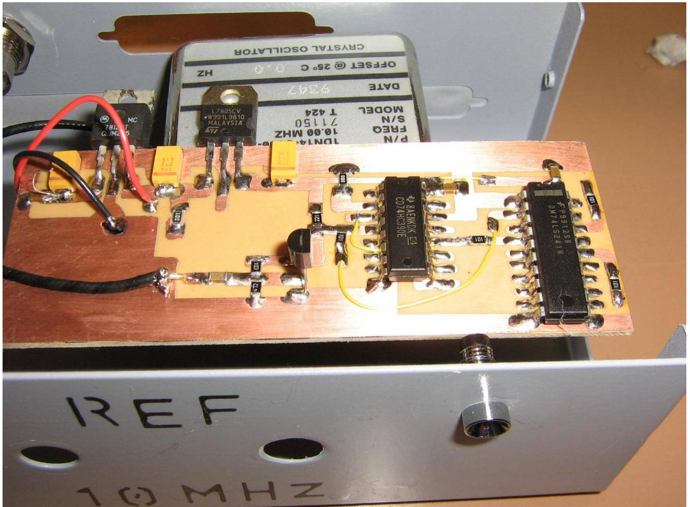
The oscillator's voltage regulator, buffer, and divider circuit board will be mounted in an old printer switch case.
