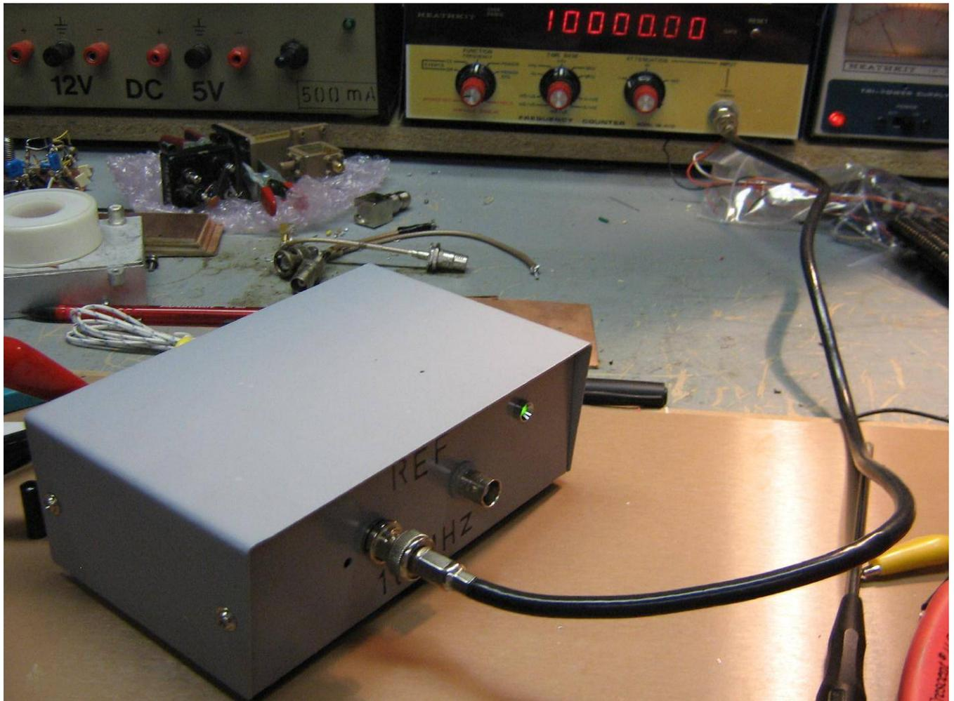
To zero-beat the oscillator, tune a shortwave receiver (AM) to the 10 MHz WWV time standard. Be sure to use a quality antenna as the received signal will need to be quite strong.
