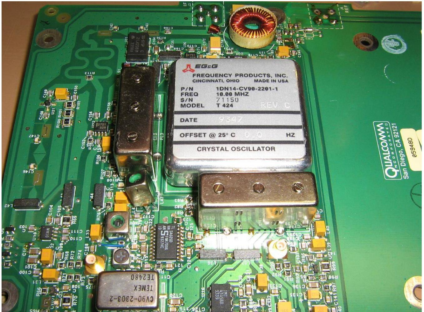
EG&G 10 MHz TCXO installed in a stock Qualcomm OmniTRACS unit.
