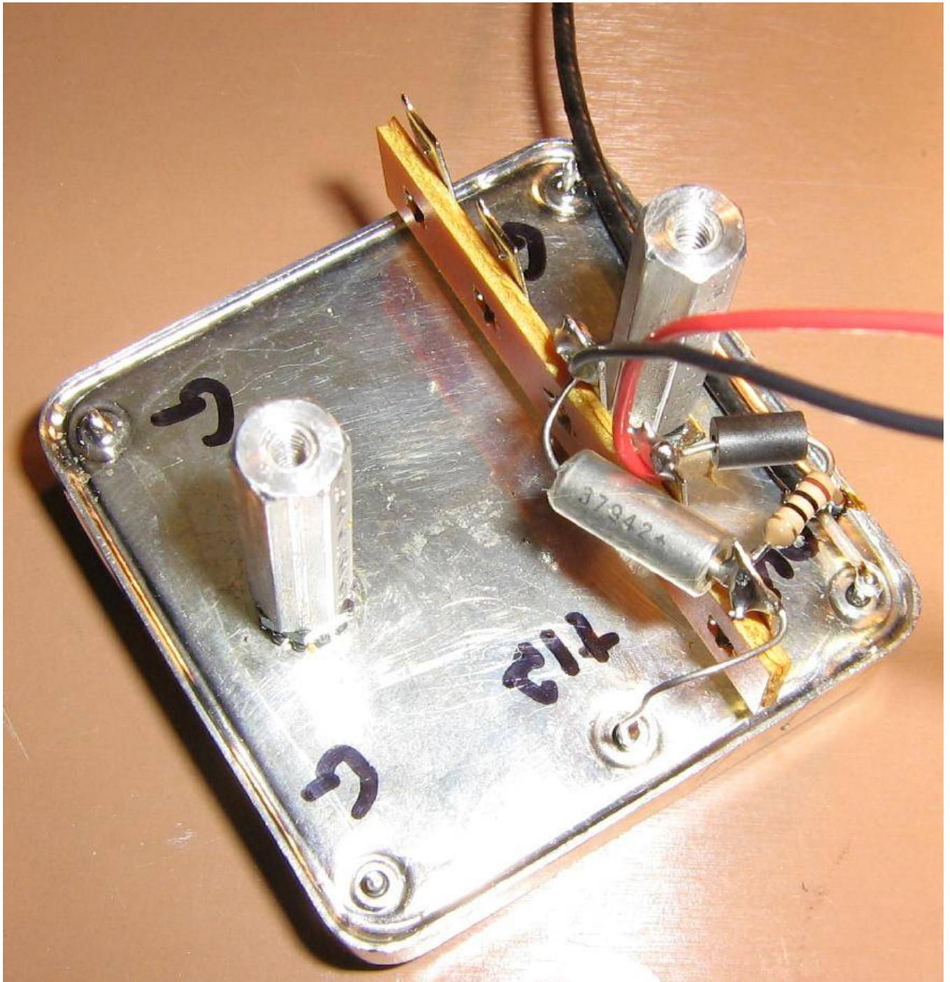
TCXO support components attached to a terminal strip.
