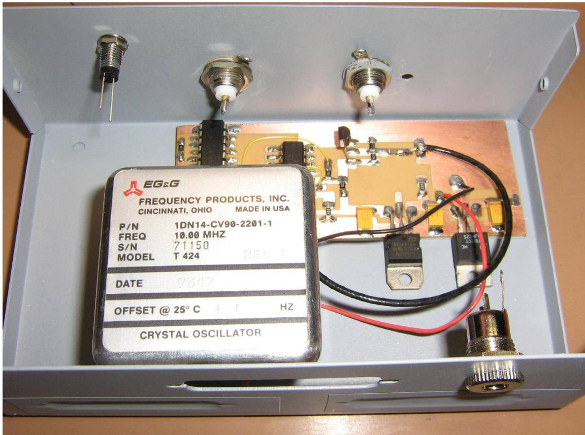
Mounting the oscillator and circuit board.
