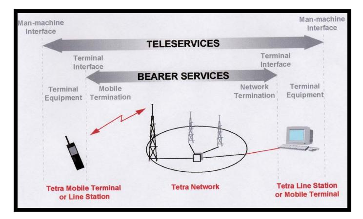
Teleservices provide complete communication capability for between users, including all terminal functions. In TETRA standards teleservices cover voice communications services. A bearer service provides communication capability between terminal network interfaces, excluding the functions of the terminal. TETRA bearer services are defined for data transfer.
