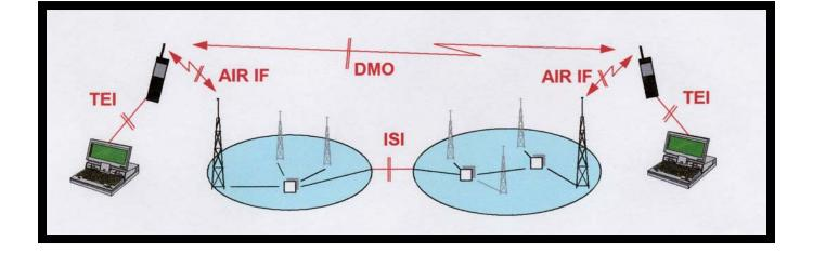
Also a line station interface is standardized. It should be noted, that the interfaces inside the Switching and Management Infrastructure are not standardized. This provides the essential benefits of an open market, but leaves the manufacturers the freedom to implement the most cost-efficient network solutions.
