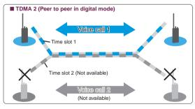
• Voice call 1 (Time slot 1) occupies whole channel, so time slot 2 stations cannot communicate.
