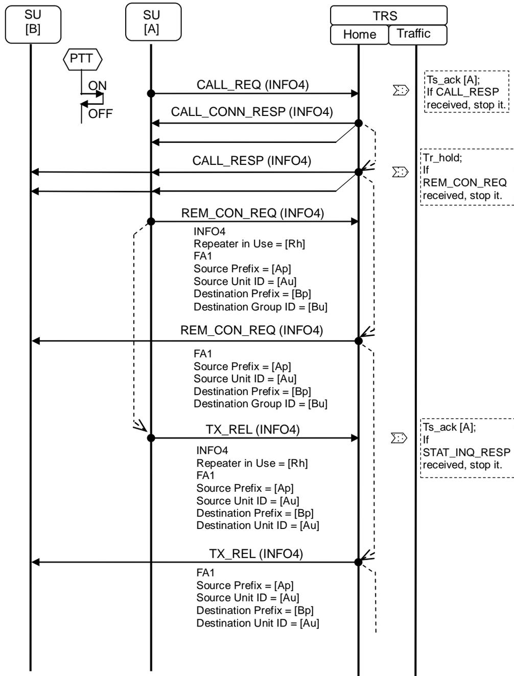
Figure 18.22-1 Sequence Diagram for Remote Stun - 1
