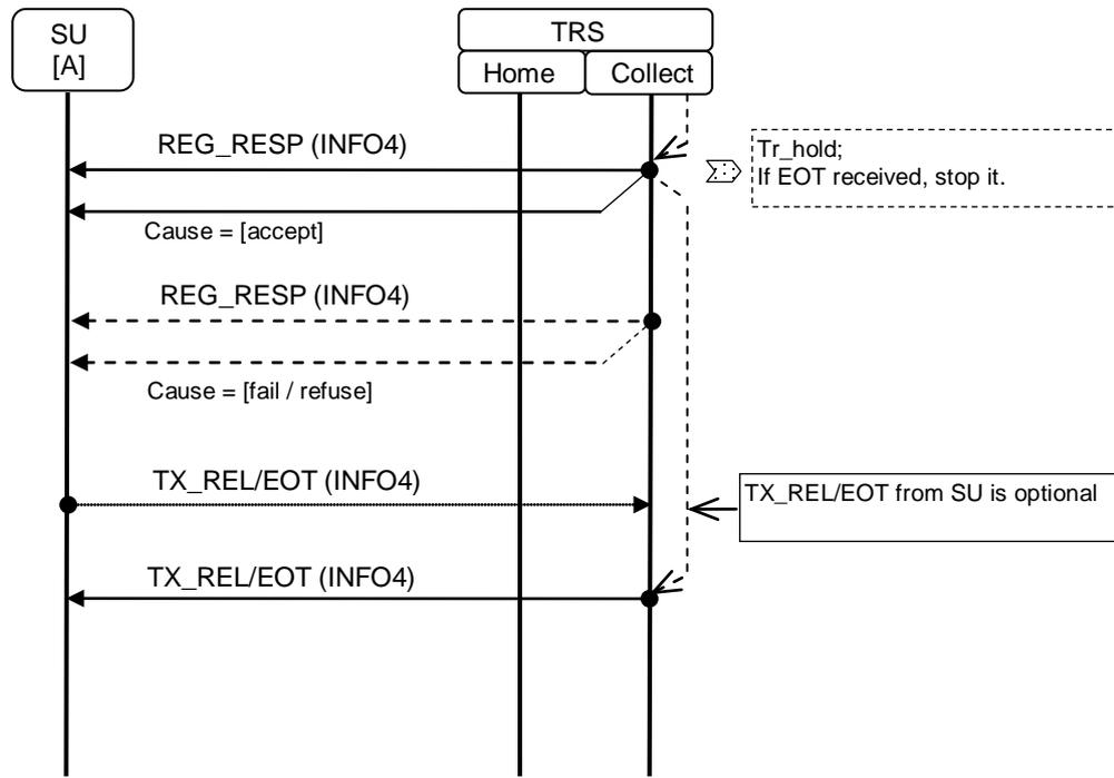
Figure 18.9-2 Sequence Diagram for System Data Write during Registration - 2
