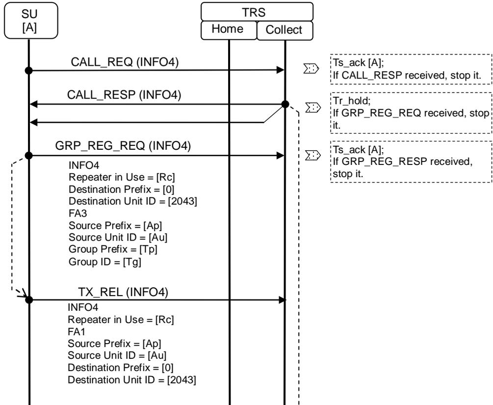
Figure 18.6-1 Sequence Diagram for Group Registration - 1
