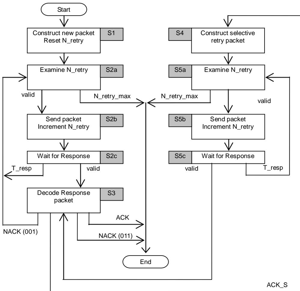
Figure 12.5-1 State diagram of confirmed packet transmission
