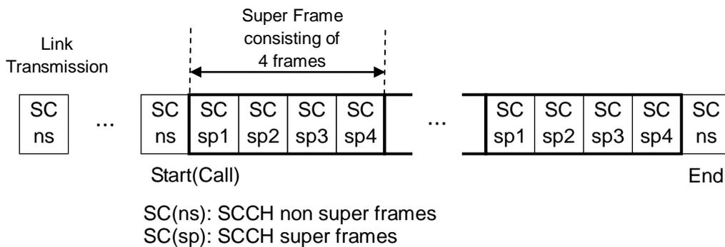
Figure 11.1-1 Frames Structure for Voice Call
