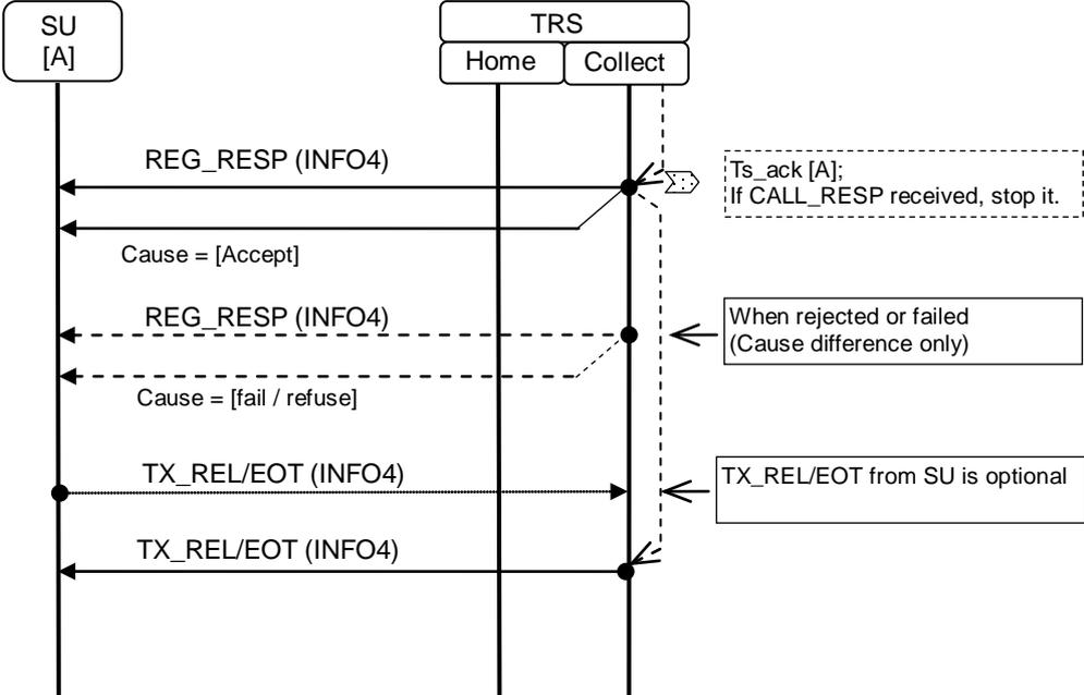
Figure 18.7-2 Sequence Diagram for Authentication during Registration - 2
