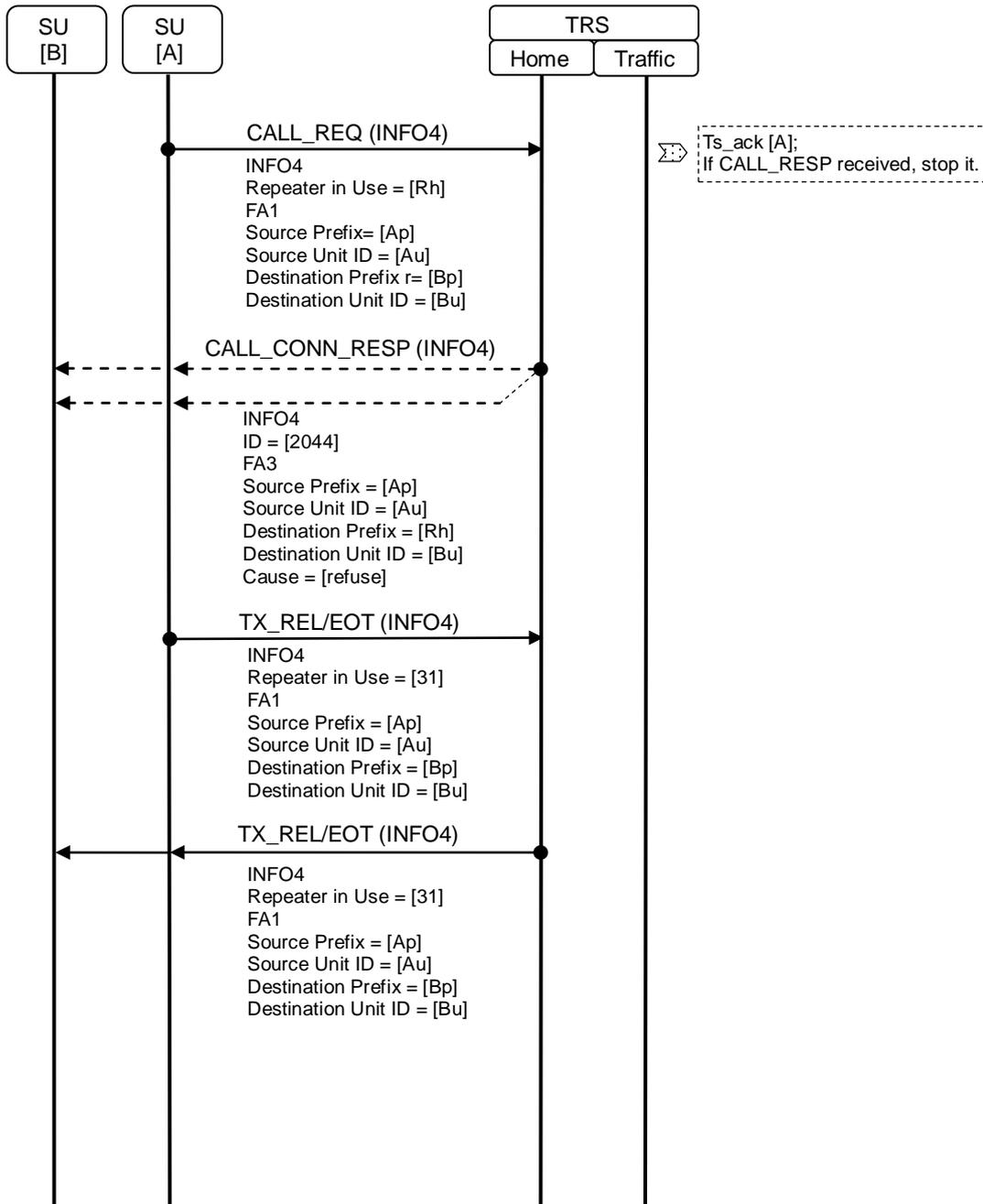
Figure 18.2-3 Sequence Diagram for Link refuse
