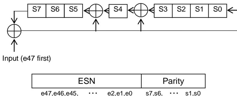
Figure 10.3-1 Parity Calculation and Bit Allocation
