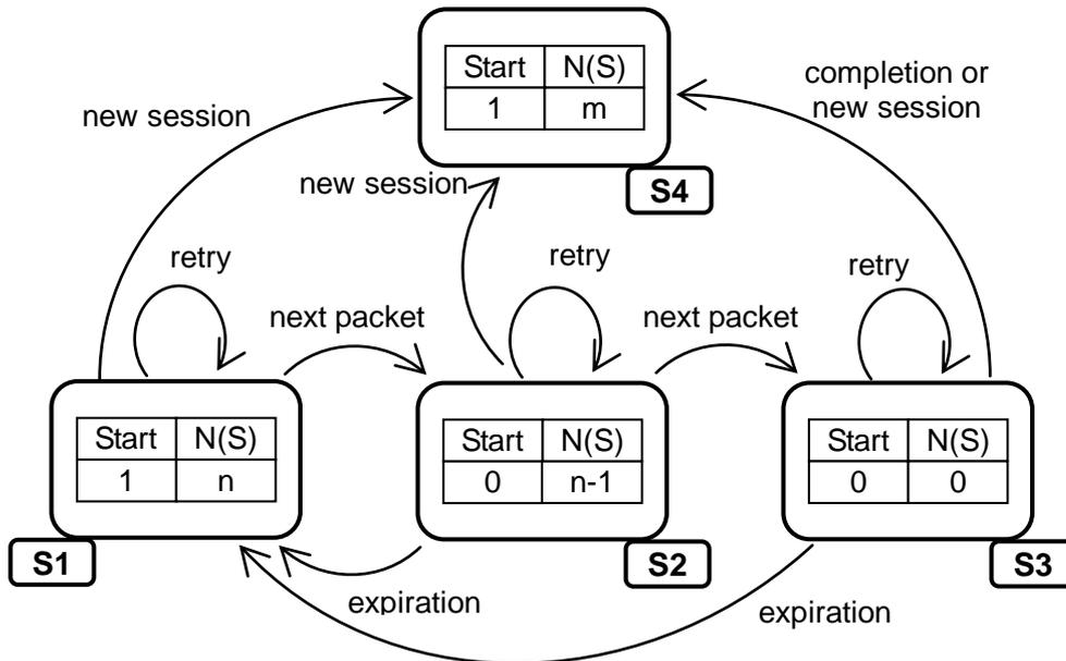
Figure 12.3-2 State transition of transmission packet
