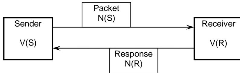
Figure 12.3-1 Conceptual diagram of packet synchronism
