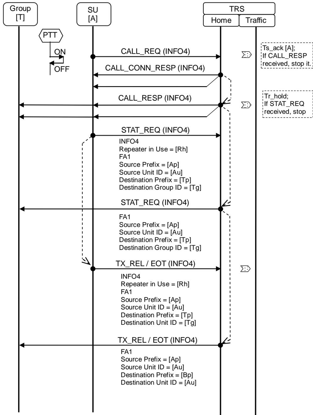
Figure 18.21-1 Sequence Diagram for Broadcast Status Call
