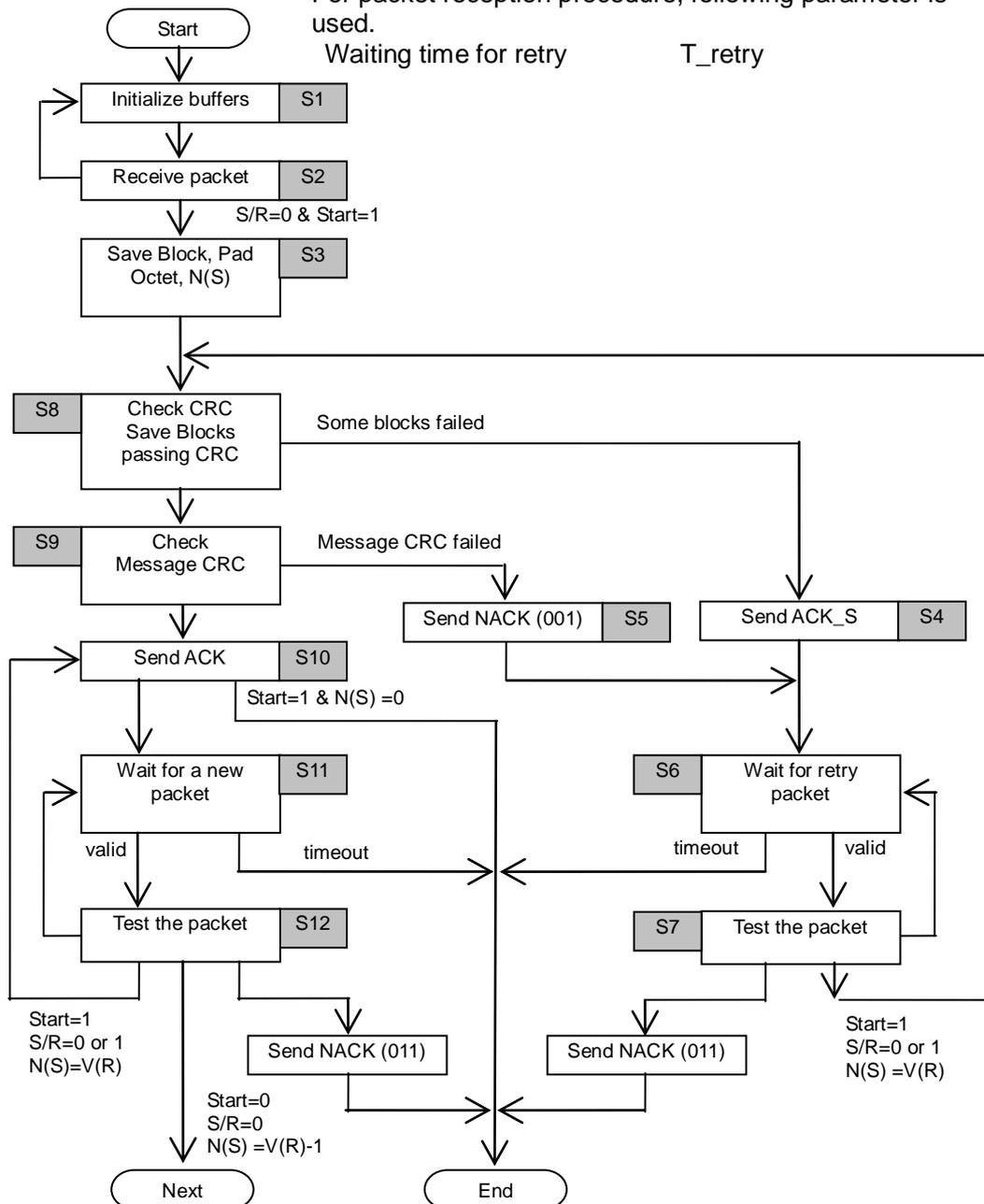
Figure 12.5-2 State Diagram of receiving the initial confirmed packet.
