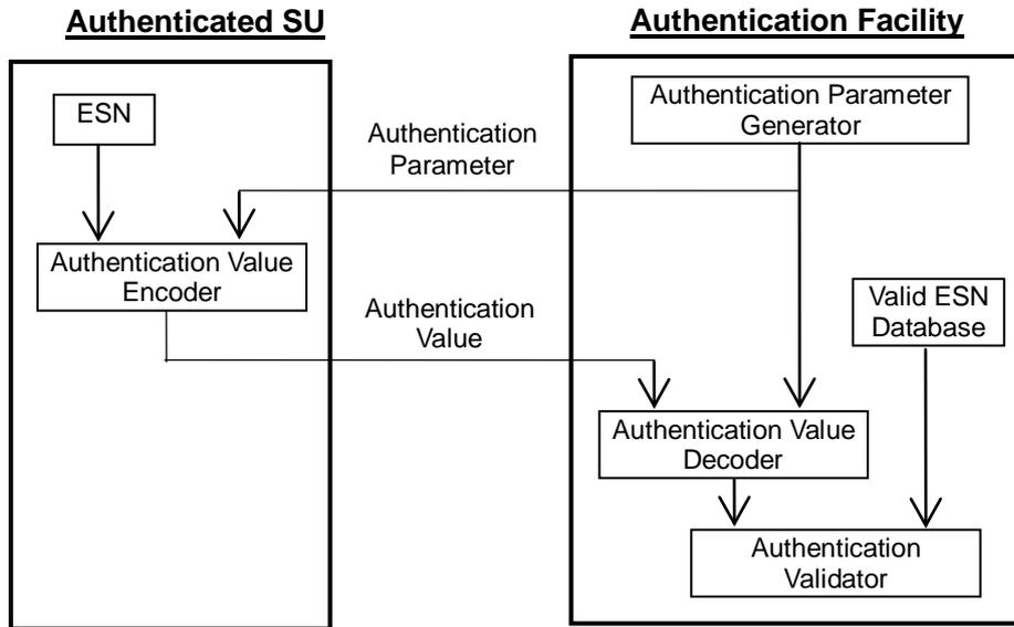
Figure 10.2-1 Block Diagram for Authentication
