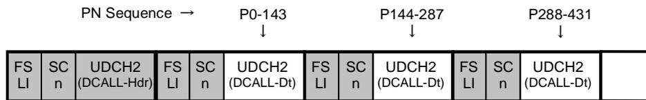
Figure 16.4-2 Relationship between PN sequence and UDCH2 in Scramble Encryption
