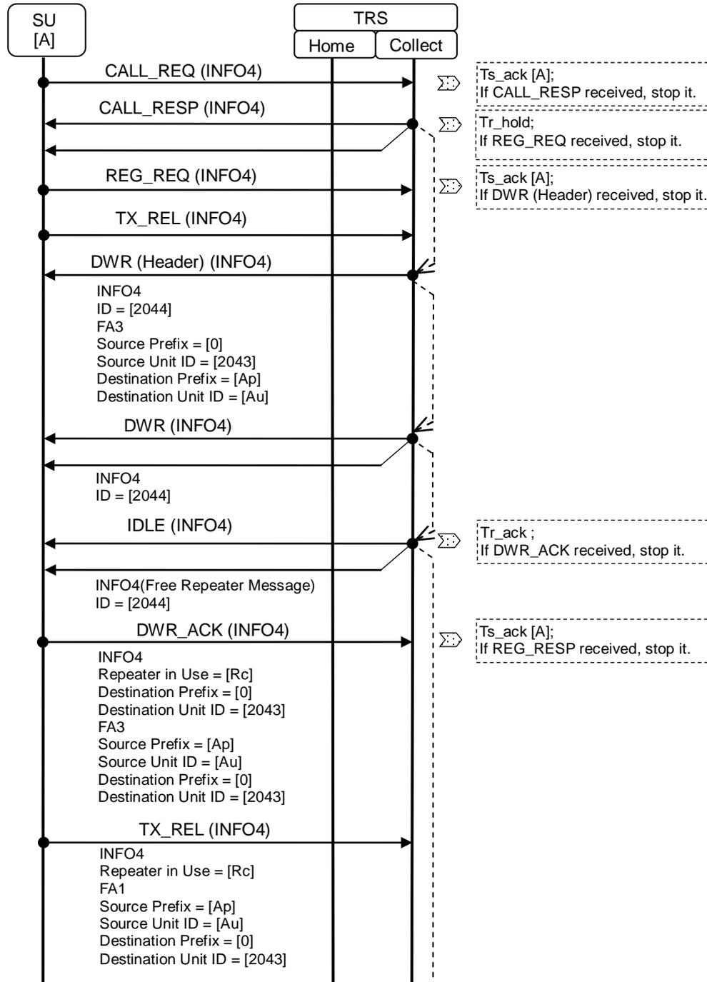
Figure 18.9-1 Sequence Diagram for System Data Write during Registration - 1
