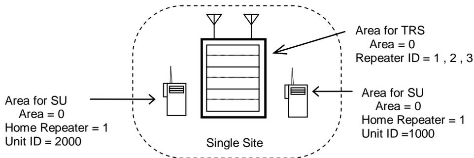
Figure 4.1-1 Concept configuration of Single Trunked System
