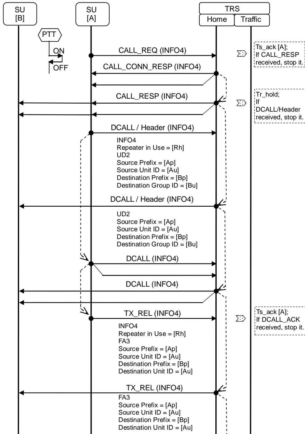
Figure 18.16-1 Sequence Diagram for Unit to Unit Data Call - 1
