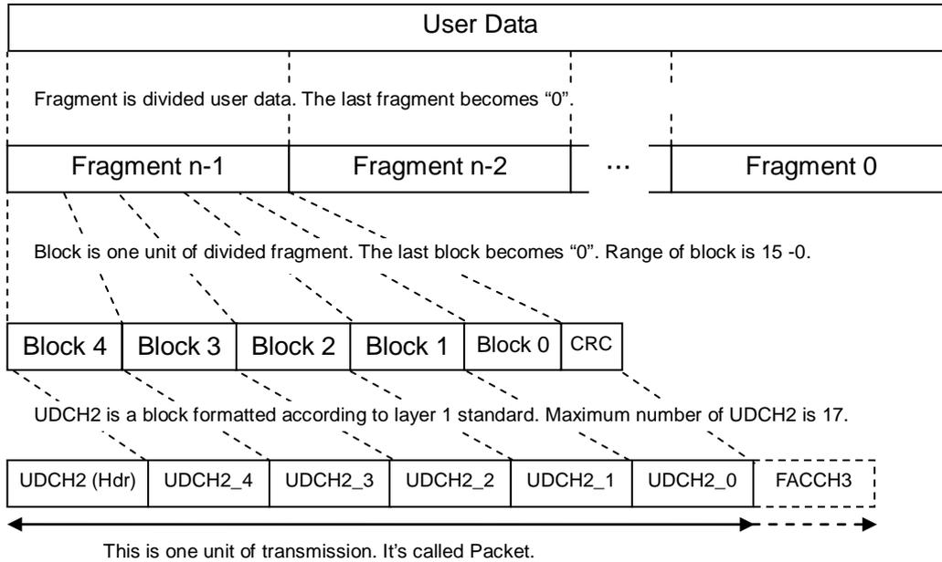
Figure 12.2-1 Concept of Data Partitioning
