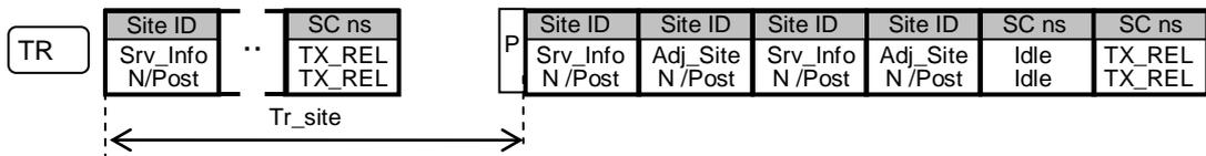
Figure 8.3-6 Transmission interval of Site ID message on Home Repeater
