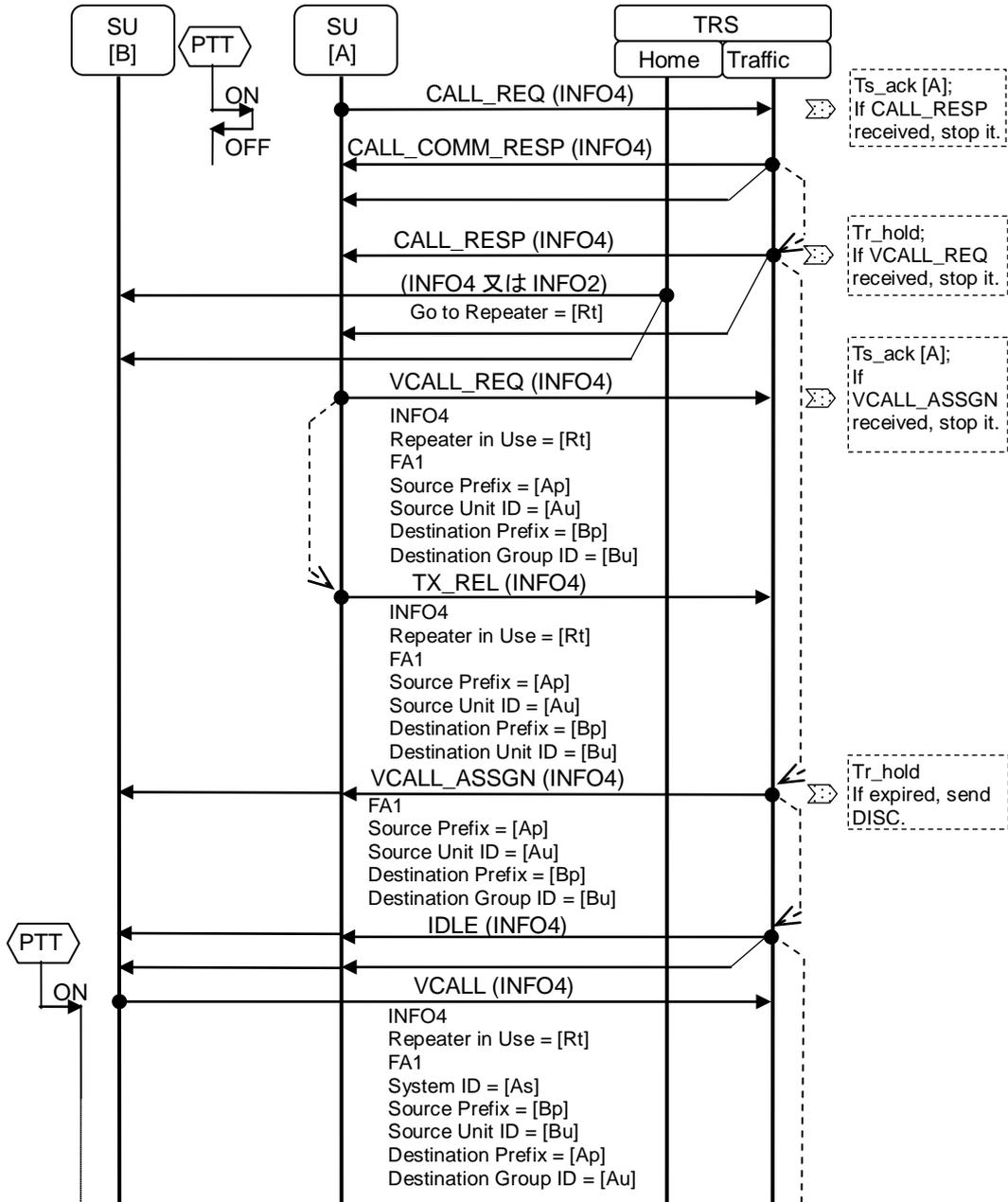
Figure 19.9-1 Sequence Diagram for Individual Voice Call - 1
