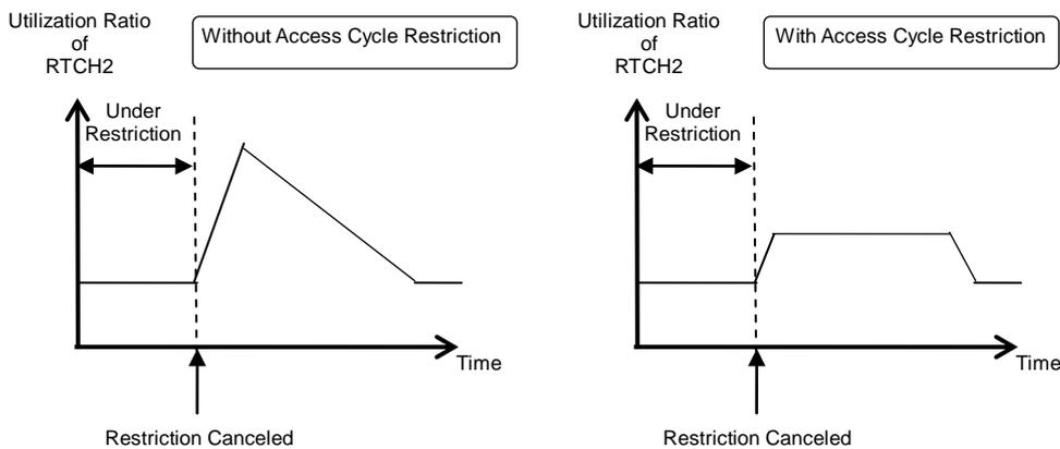
Figure 19.7-2 Utilization Ratio of RTCH2 when Access Restriction is Canceled
