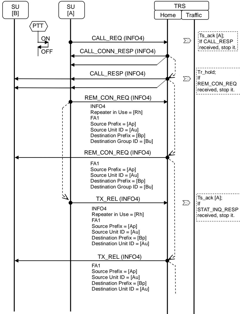
Figure 18.23-1 Sequence Diagram for Remote Monitor – 1
