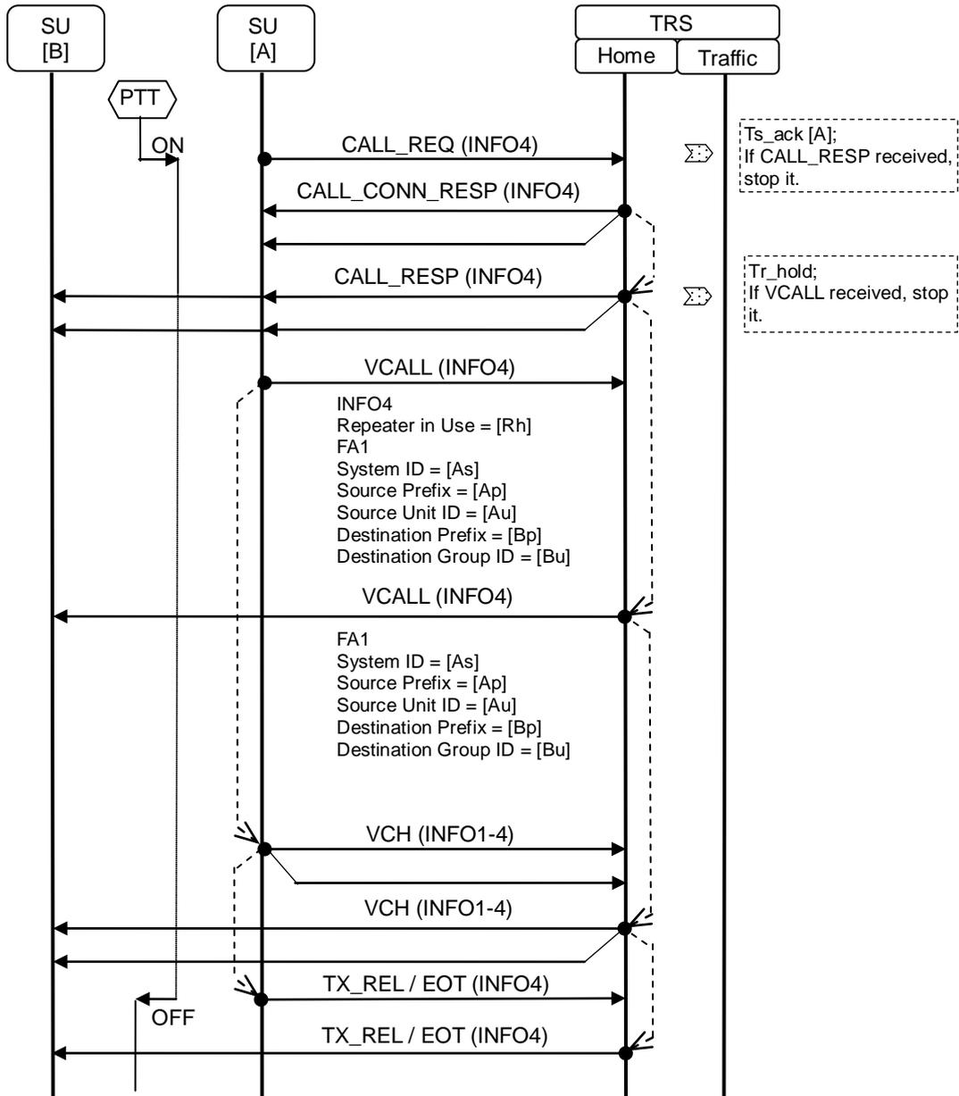
Figure 18.12-1 Sequence Diagram for Individual Call by Transmission Trunked Mode
