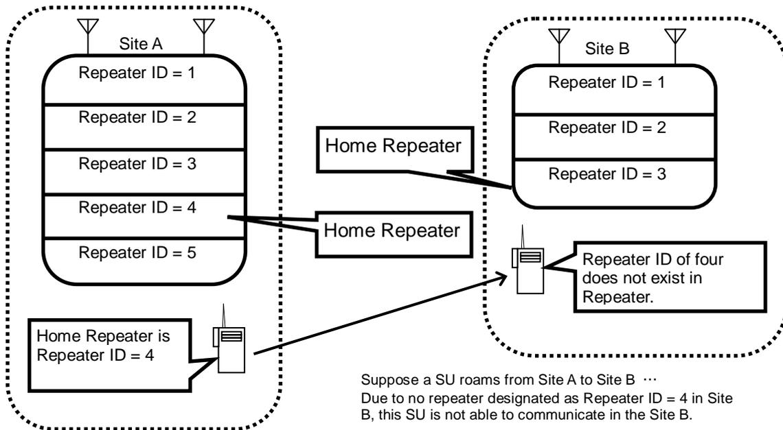
Figure 5.1-1 In the case where a Repeater ID indicating a Home Repeater is allocated:
