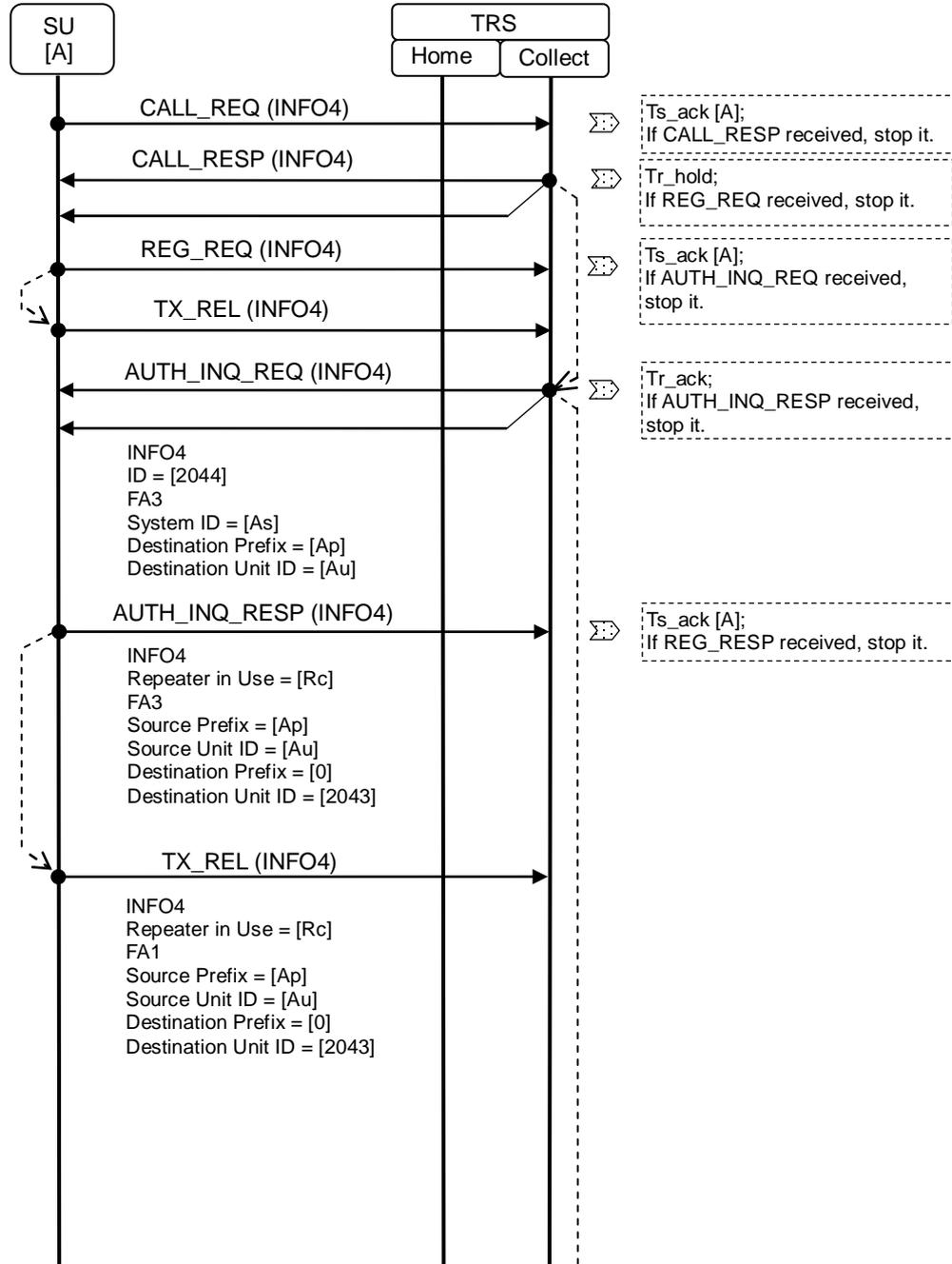
Figure 18.7-1 Sequence Diagram for Authentication during Registration - 1
