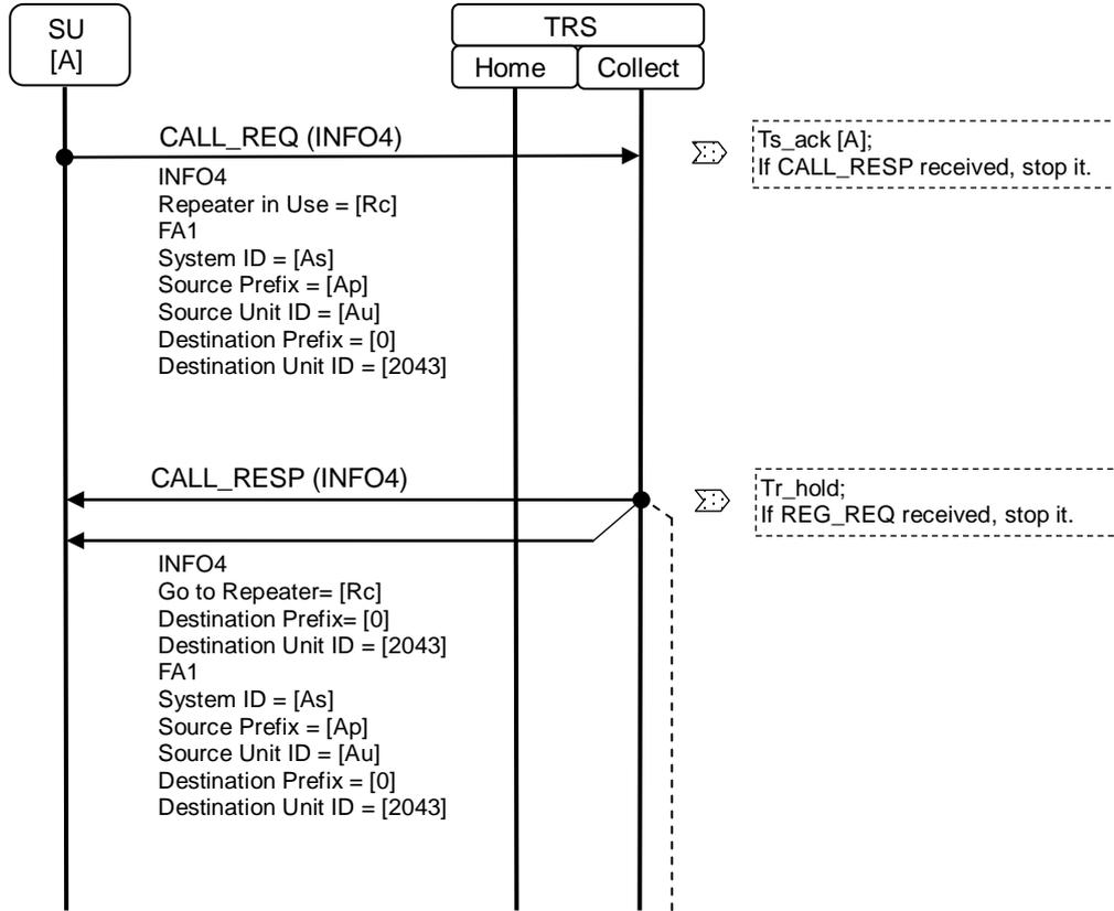
Figure 18.3-1 Sequence Diagram for Registration - 1
