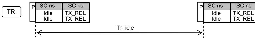
Figure 8.3-4 Transmission interval of Idle message
