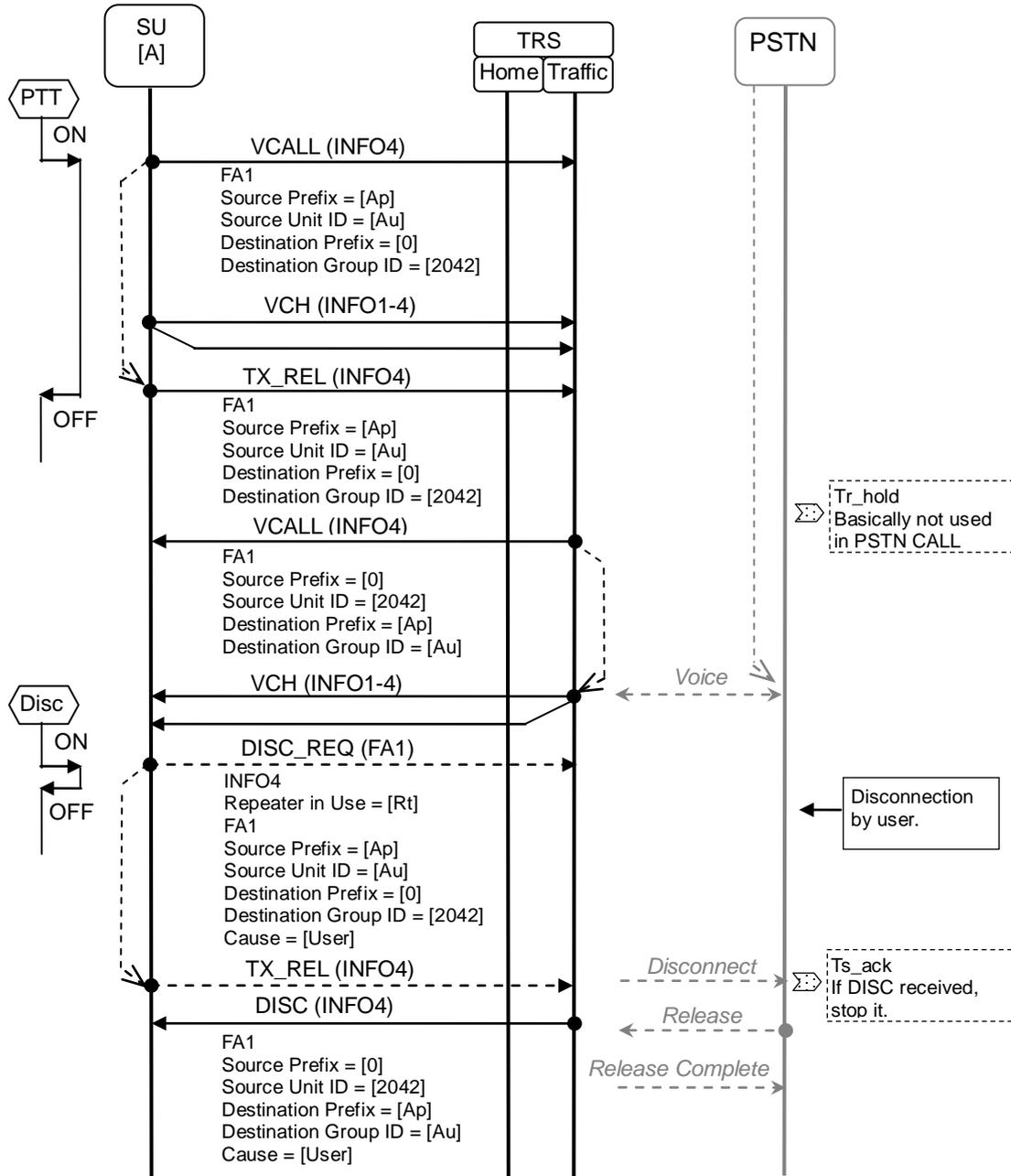
Figure 18.13-2 Sequence Diagram for Unit to PSTN Voice Call – 2
