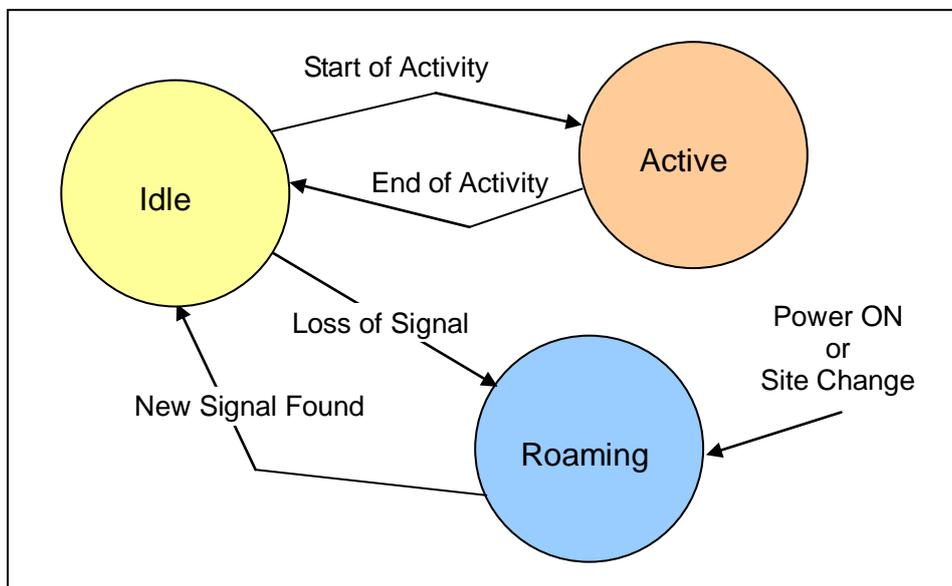
Figure 6.1-1 Basic Data Flow for Roaming Process
