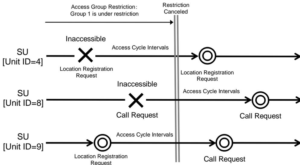
Figure 19.7-3 SU Behavior under Access Cycle & Access Group Restriction
