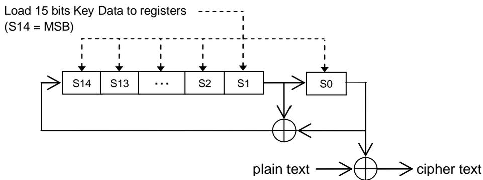
Figure 16.3-1 Scramble Encryption Algorithm
