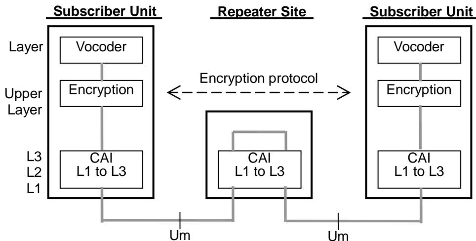
Figure 16.1-1 Layer for Encryption Protocol
