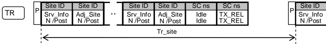
Figure 8.3-5 Transmission interval of Site ID message on Collect Repeater
