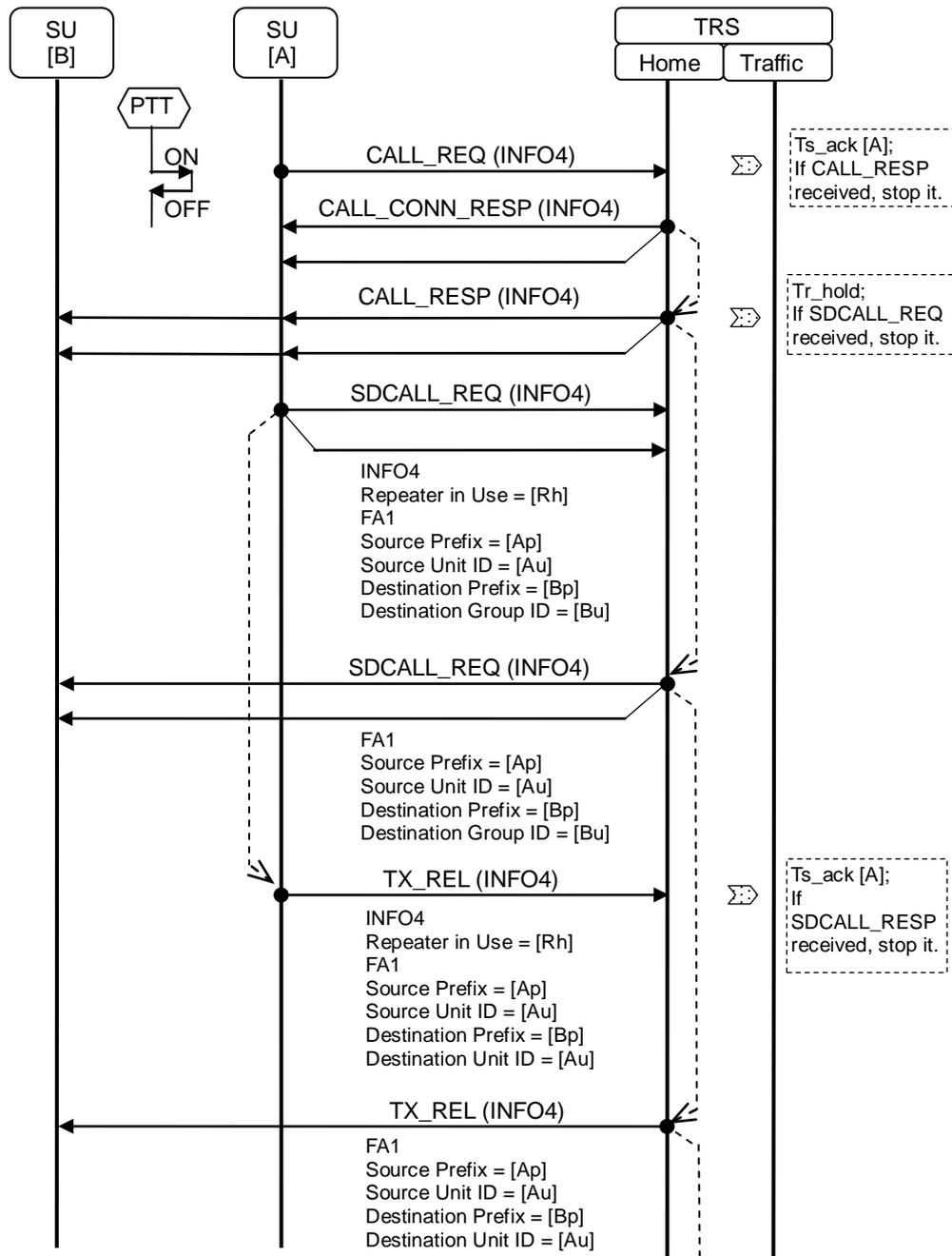
Figure 18.18-1 Sequence Diagram for Unit to Unit Short Data Call - 1
