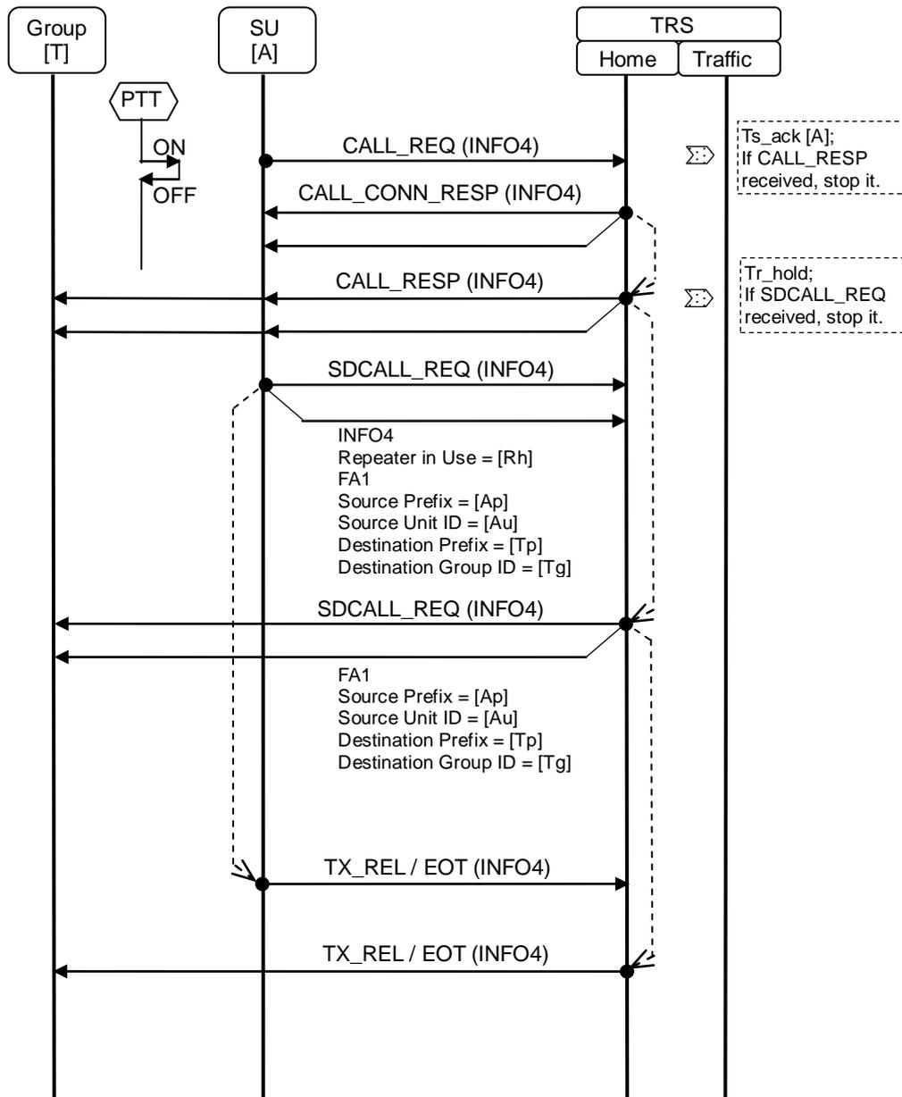
Figure 18.17-1 Sequence Diagram for Broadcast Short Data Call
