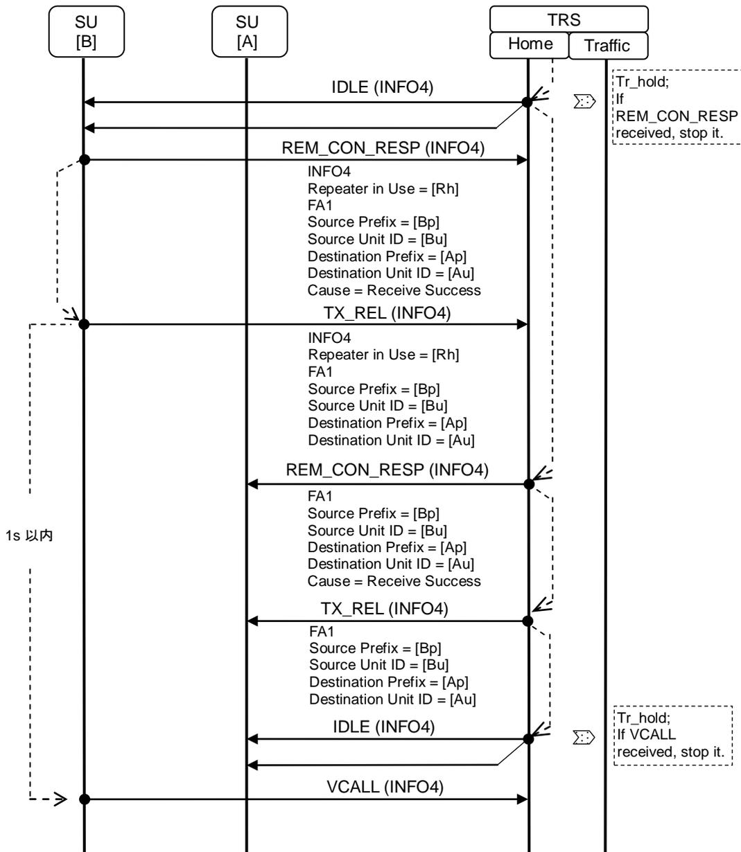
Figure 18.23-2 Sequence Diagram for Remote Monitor - 2
