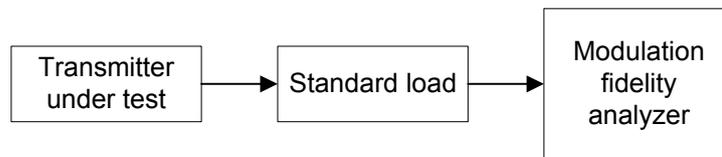
Figure 5.2-11 Modulation Accuracy
