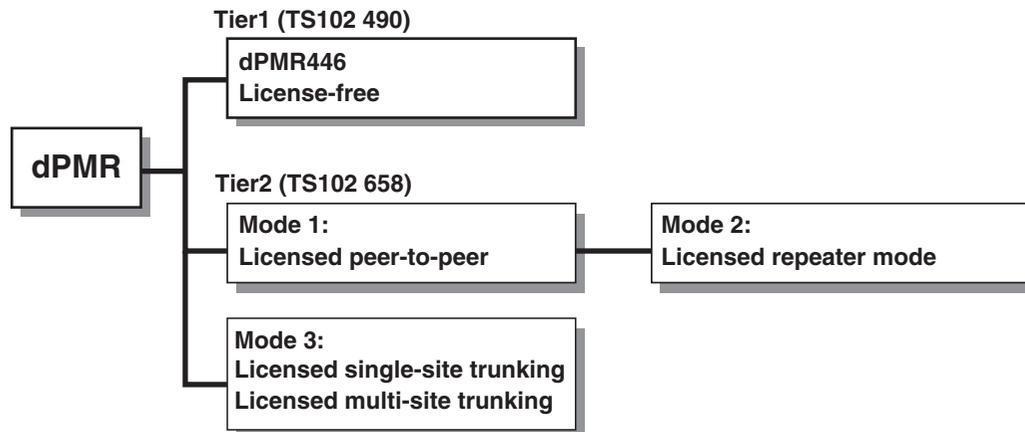
As the diagram shows, dPMR™ is a full featured system capable of providing communications solutions ranging from license-free all the way up to nation-wide networks. The main difference to NXDN™ is additions of the license-free standard. The dPMR™ protocol allows for system sizes up to a potential of 1,000 sites and millions of users.
