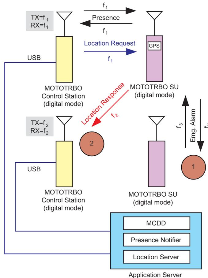
Figure 4-27 Emergency Alarm and GPS Revert Interaction Diagram
