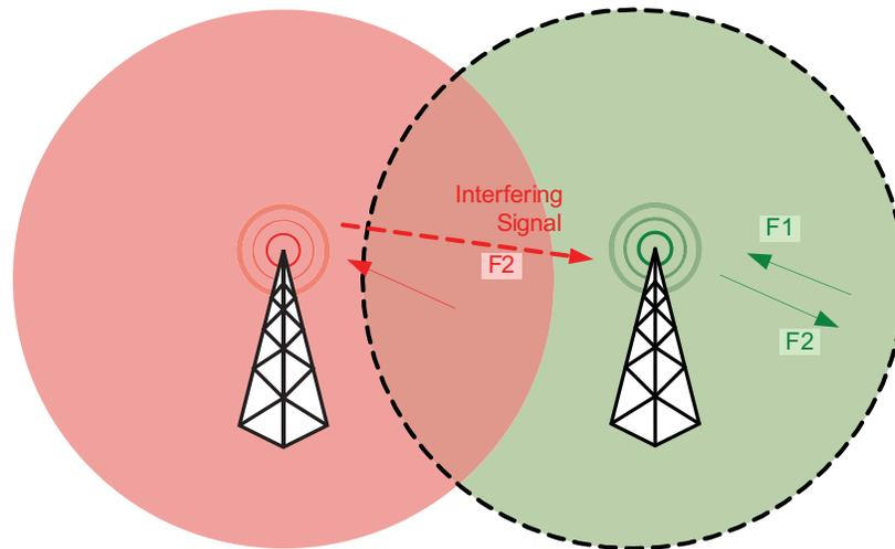
*Figure 4-21 An Example of Interference at Transmit Frequency*
