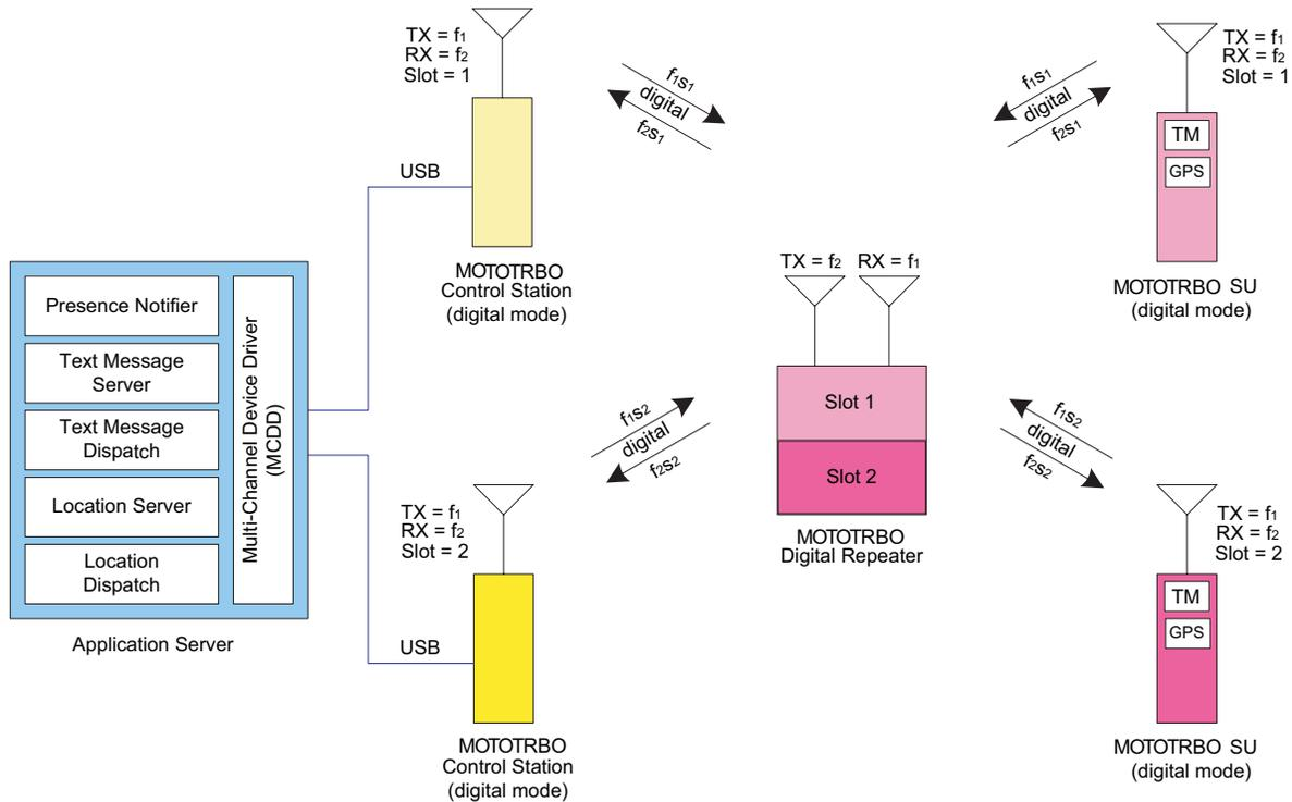
Figure 3-23 MOTOTRBO Radios in Digital Two-Slot Digital Repeater Mode with a Server-Based Configuration
