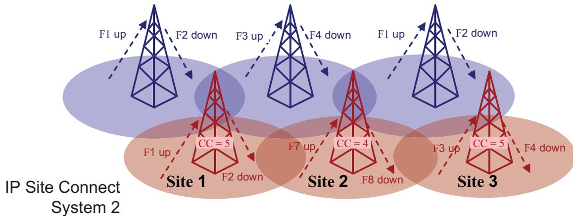
Figure 4-17 Example of Two IP Site Connect Systems with Overlapping Coverage Areas
