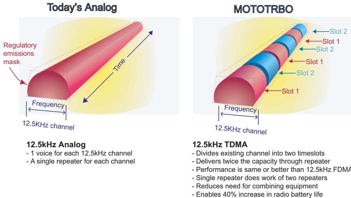
*Figure 2-2 Comparison between Today's Analog and MOTOTRBO*
