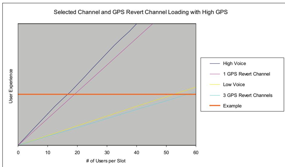
Figure 4-6 Channel Loading with GPS Revert Channels
