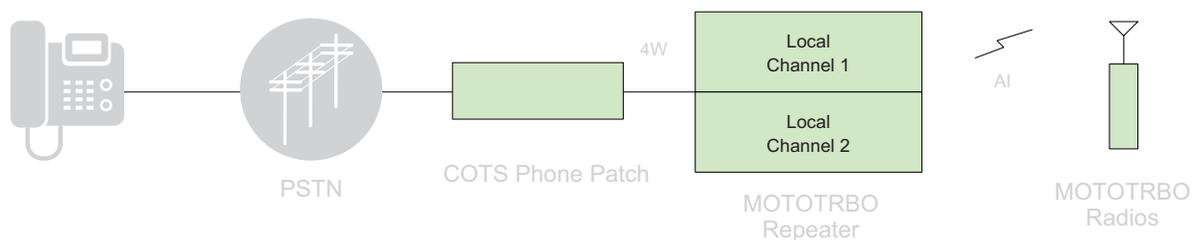
Figure 2-20 Phone Patch Topology in Single Site Configuration
