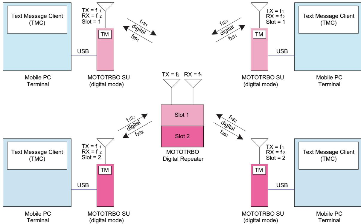
Figure 3-21 MOTOTRBO Radios in Digital Two-Slot Digital Repeater Mode with Text Messaging
