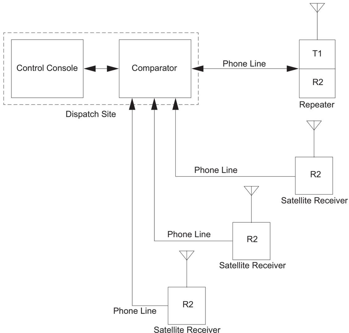
Figure 3-1 Satellite Receiver Connections Within a Voting System
