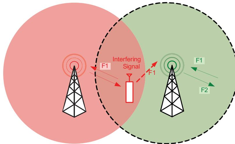
Figure 4-20 An Example of Interference at Receive Frequency
