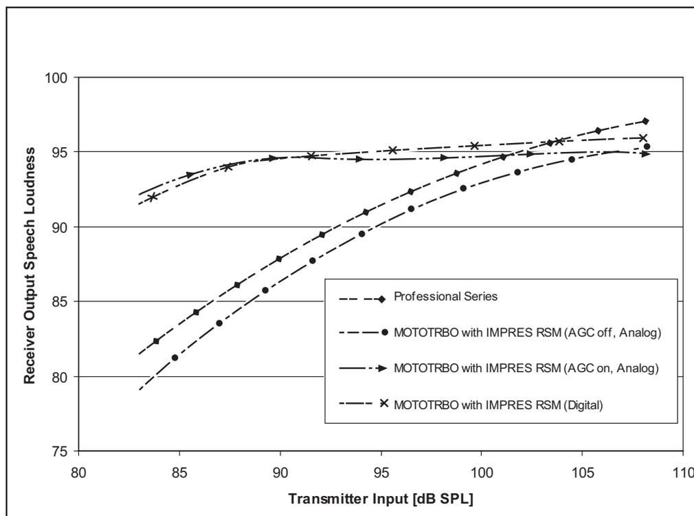
Figure 2-7 Transmit Audio Sensitivity
