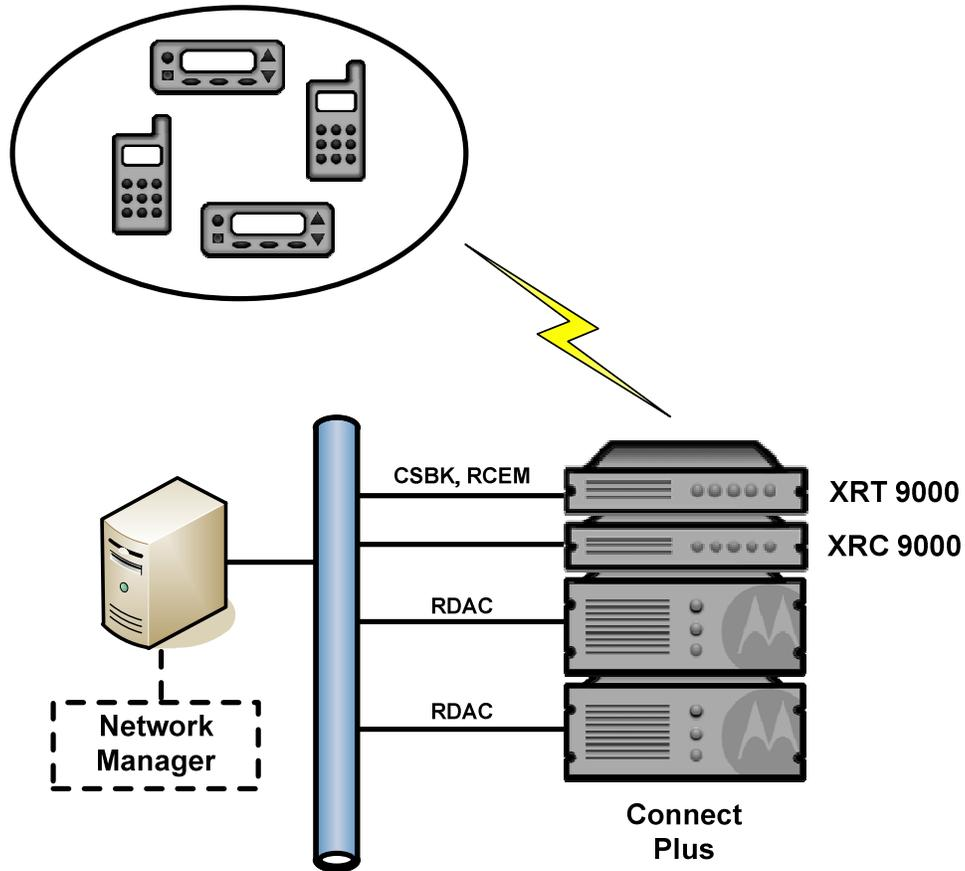
Figure 4-5 Typical Network Management Solution Topology Example for Controller-based Systems
