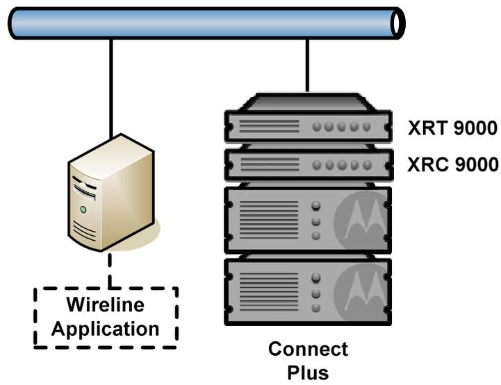
Figure 3-2 Wireline Application Topology for Controller-based Systems
