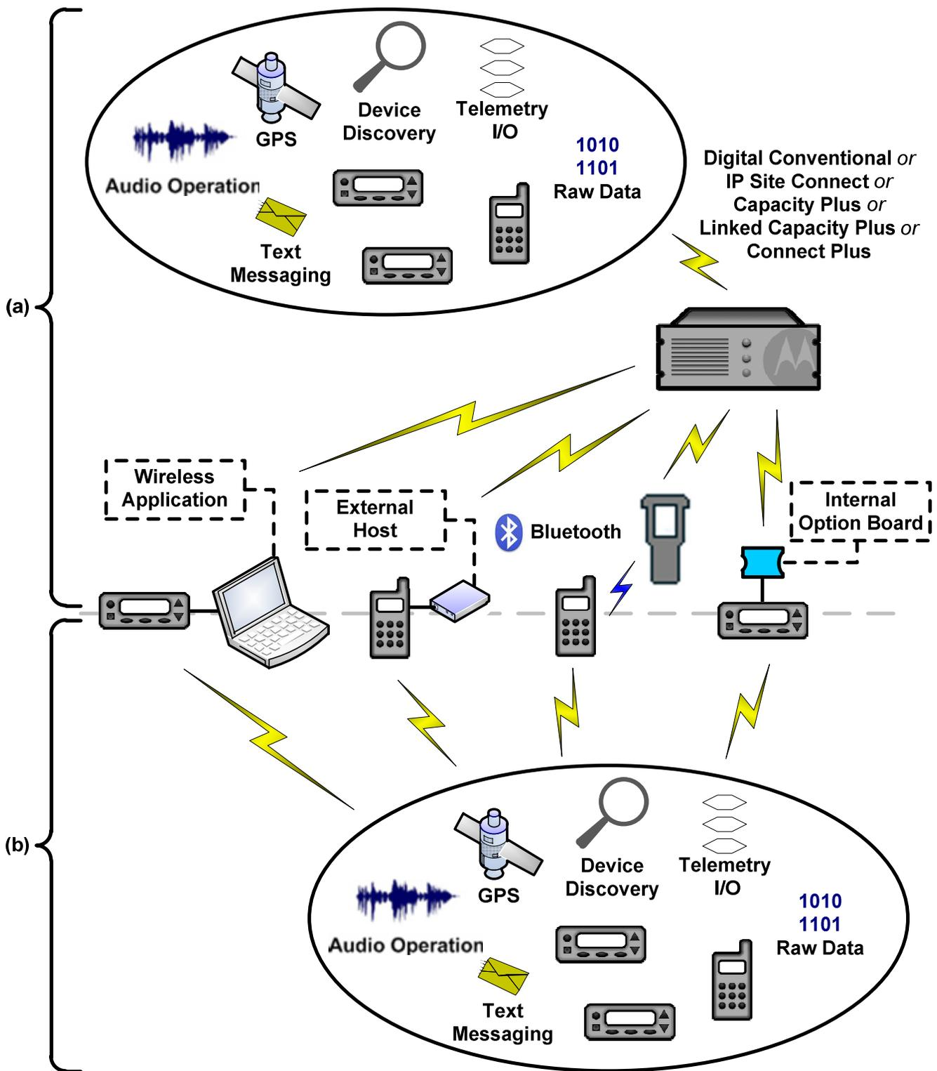
Figure 4-3 Interoperability Examples of Radio Control Solution Topologies –
