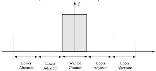
The requirements of EN 301 166 call for 60dB protection for the next 6.25 kHz channel and 70dB protection for the next channel.
