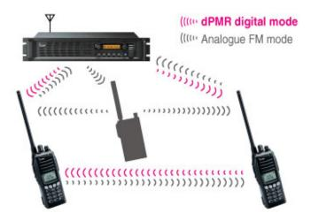
Backwards compatibility to analogue only radios enables a planned migration path to "digital" with existing radios operating analogue only and new radios operating analogue and digital.
