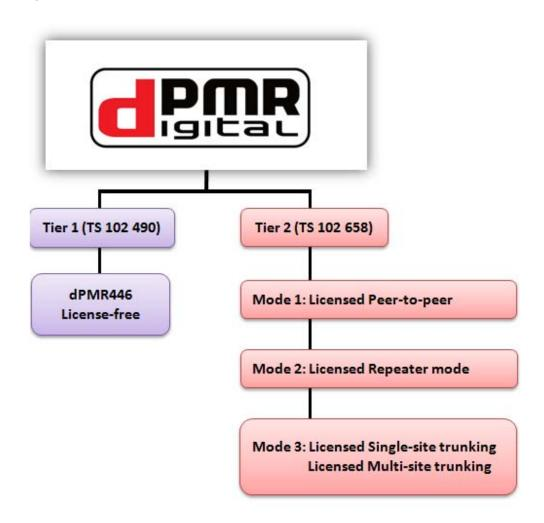
As the diagram shows, dPMR<sup>™</sup> is a full featured system capable of providing communications solutions ranging from license-free all the way up to multi-site trunking networks.
