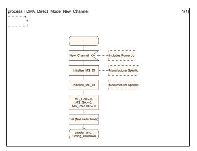
Figure 6.2: Power up and channel change SDL
