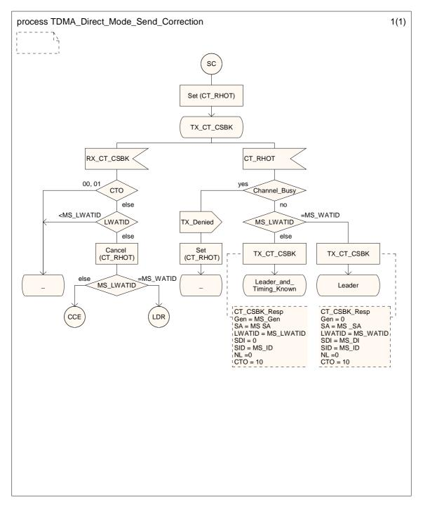
Figure 6.9: Send correction SDL
