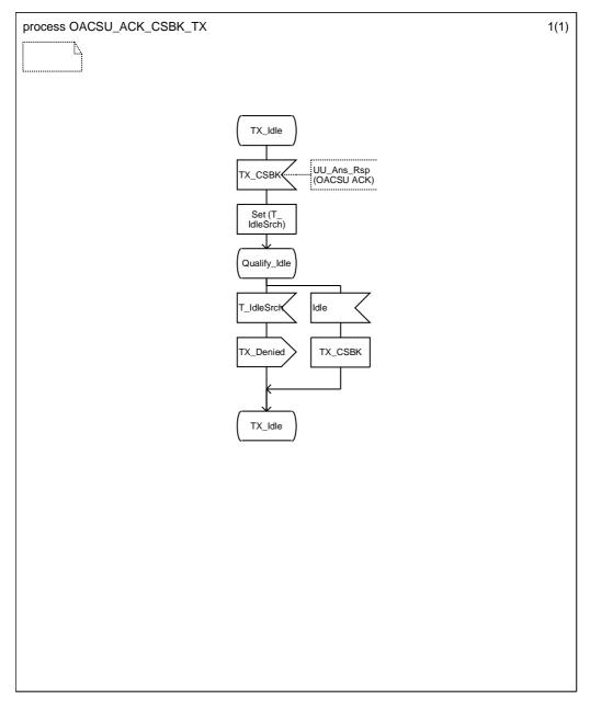
Figure 5.23: UU\_Ans\_Rsp Channel Access SDL
