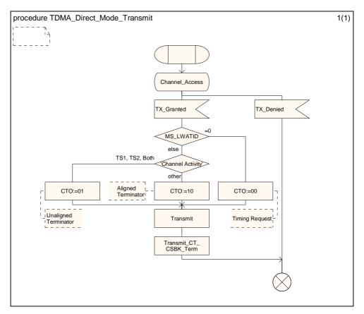
Figure 6.13: Transmit procedure SDL
