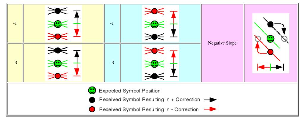
All three tracking loops run once every symbol time period with no unpleasant interactions. Lock in occurs over a broad range of gain variables. The gains as implemented in the sample code have been chosen for rapid signal acquisition of the symbol sync sequence ( $\sim$ 16 symbols repeating a +3, +3, -3, -3, pattern transmitted whenever the transmitter is keyed up).
