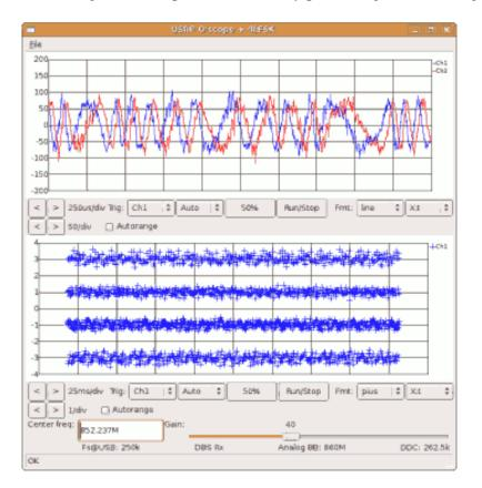
Live graphs are neat. Here we have the incoming data signal on top and the demodulator block output on the bottom. 4L-FSK demodulator performance can be assessed immediately - you should see a set of nicely separated data symbols as in the example above (after setting the graph format to "plus" style). This real time display is quite handy for optimizing the system.
