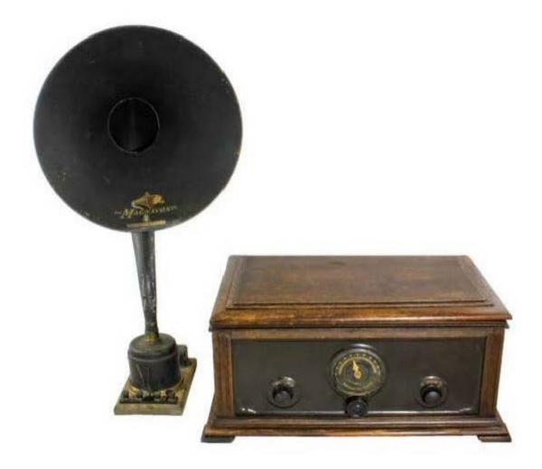
In 1923, Magnavox invented the world's first single-dial radio. The radio, TRF-5, is shown with the R3 speaker. The set used 2 RF and 2 Audio amplifier (type A) tubes, plus 1 detector tube (type D), A&B batteries and covered the AM broadcast band.
