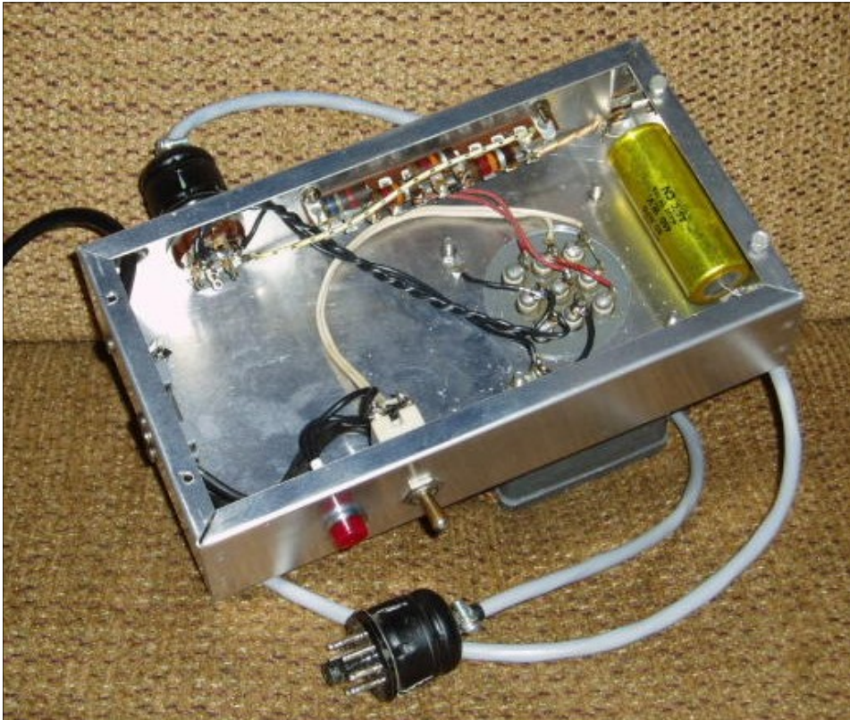
Inside Power Supply Chassis
