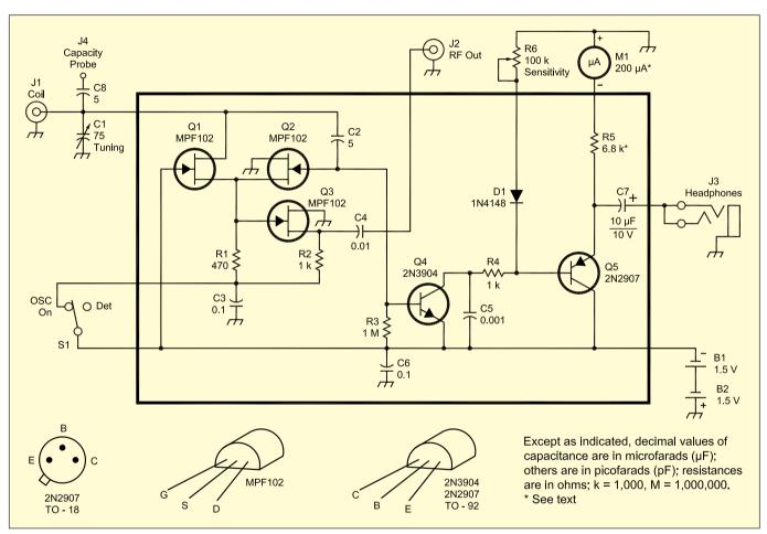
Figure 4—Schematic diagram of the GDO. Part numbers listed are from Ocean State Electronics (OSE) (800-866-6626, www.oselectronics.com), Alltronics (408-847-0033, www.alltronics.com), Digi-Key (800-344-4539, www.digikey.com) and Mouser Electronics (800-346-6873, www.mouser.com). Resistors are available from all of the above sources.
