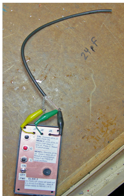
Photo 6 shows the L-C meter and the coax capacitor connected. The L-C meter outputs the value in Morse Code.
