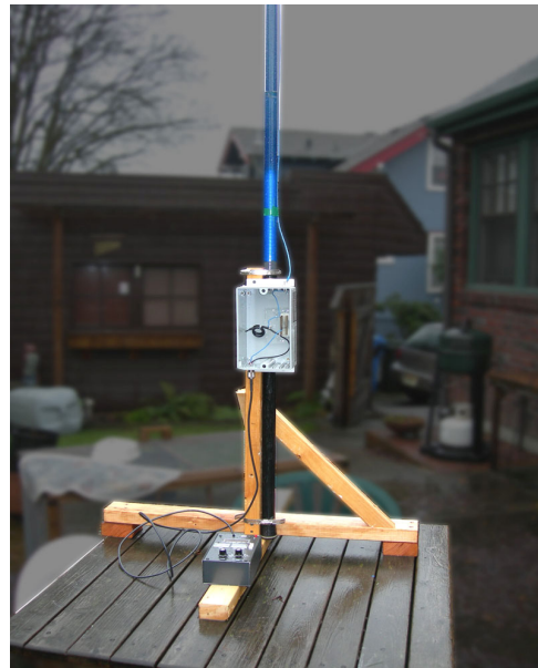
Photo 8 Final assembly: Plastic enclosure connected to wooden stand and fiberglass fishing pole connected to stand.
